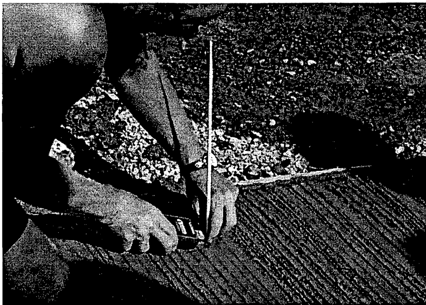
Figure 4: Maturity probe insertion into newly placed PCC
