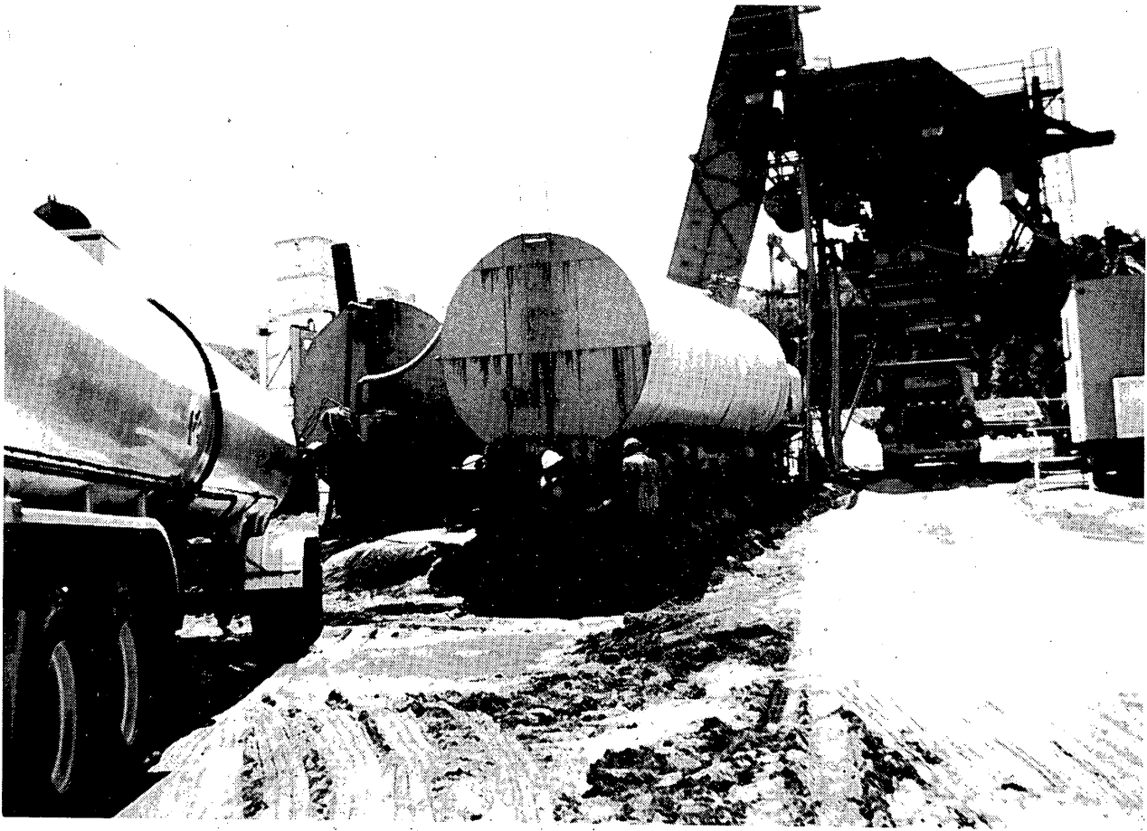
Figure 1 - Cedar Rapids Batch Plant With Dual Storage for Two Sources of Asphalt Cement
