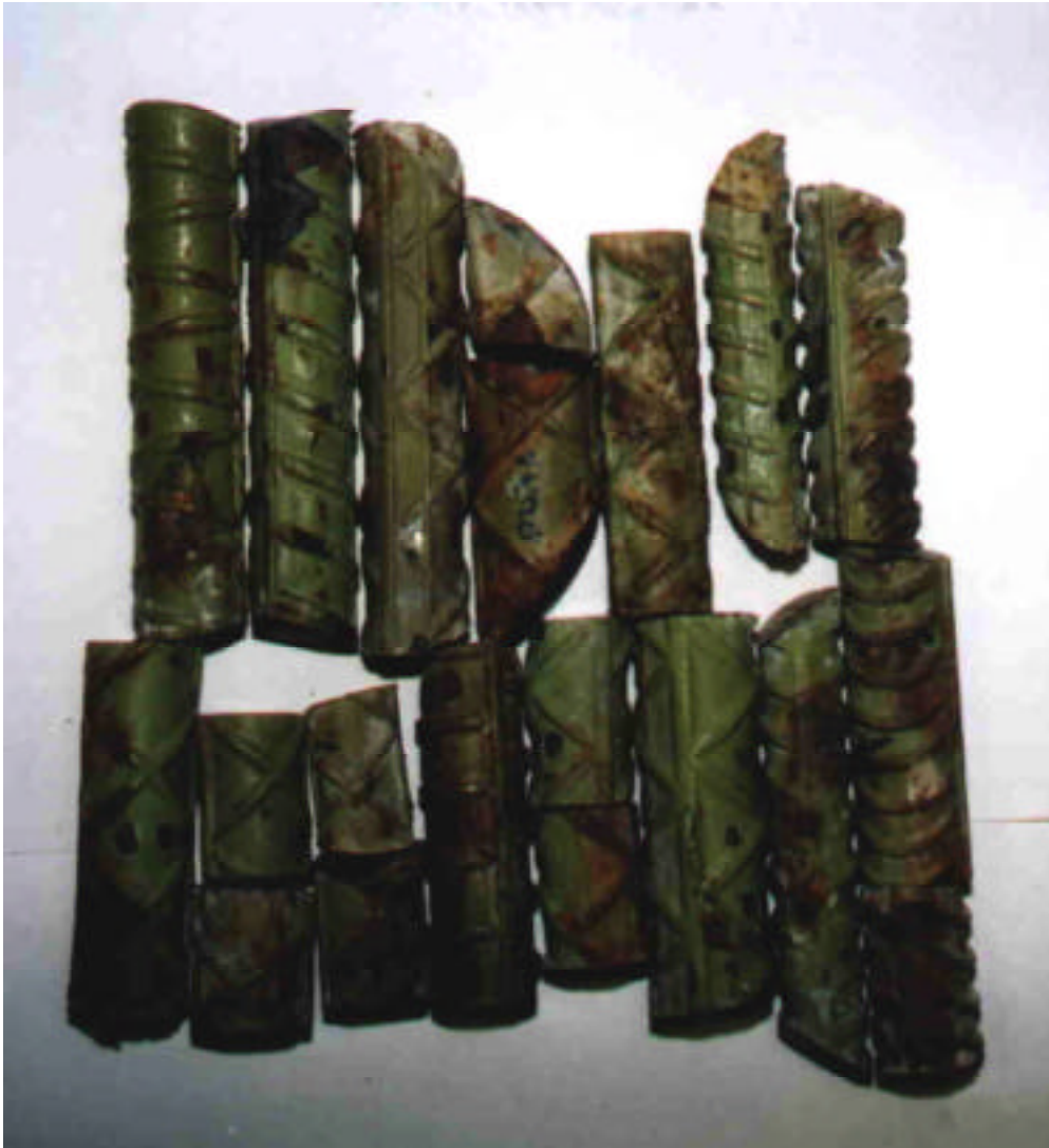
FIGURE 6.3 Rebars Samples with Significant Corrosion
