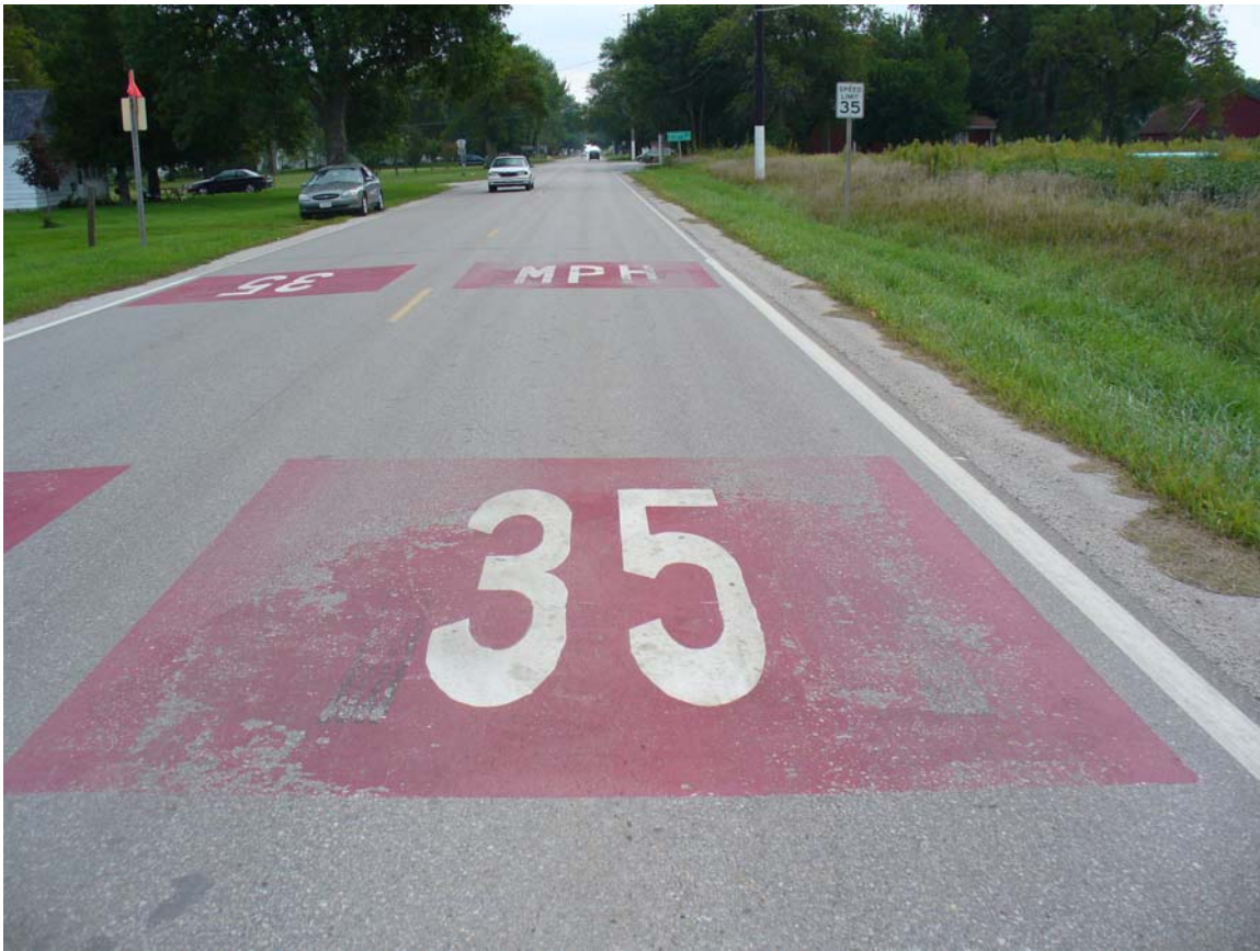
Figure 5.45. Wear of Dexter treatment over time.
