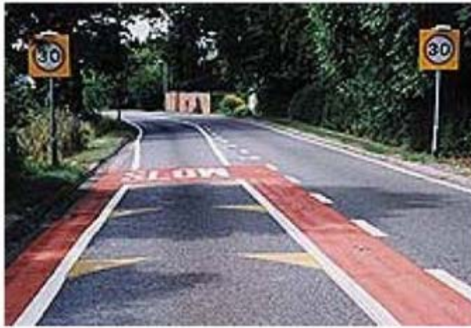
Figure 3.25. Red markings with posted speed limit signs (source: DETR 2005)
