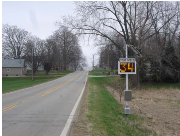
Figure 5.9. Feedback sign with driver's posted speed
