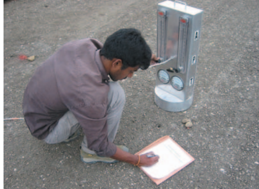
Air Permeater Test (APT) device
