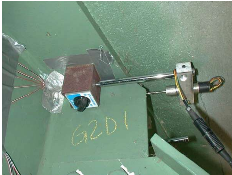
a. G2 out-of-plane displacement transducer looking west.
