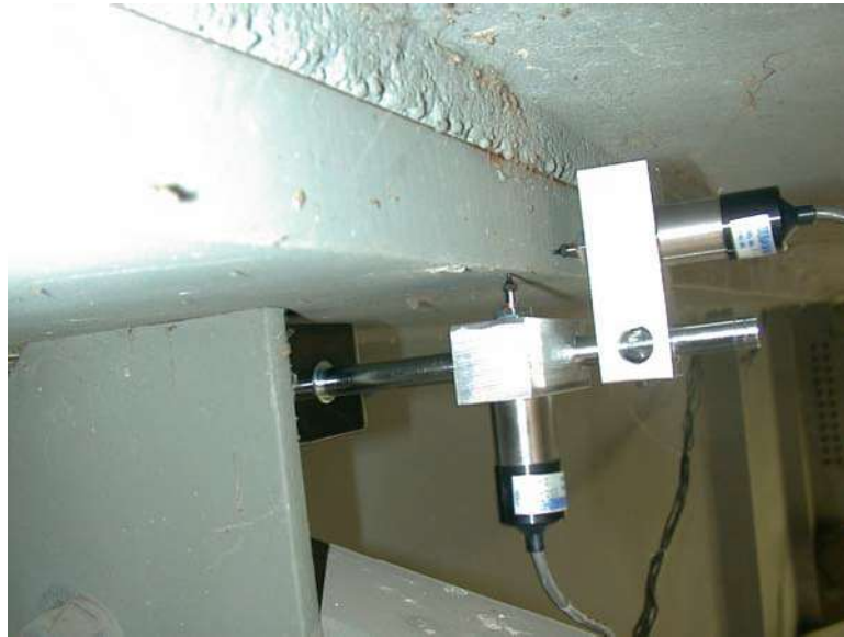
a. Photograph of out-of-plane and tipping transducers.
