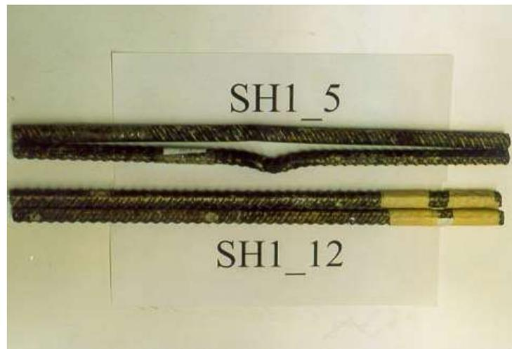
Figure 5.18. Reinforcing bars from specimens SH1-5 and SH1-12.
