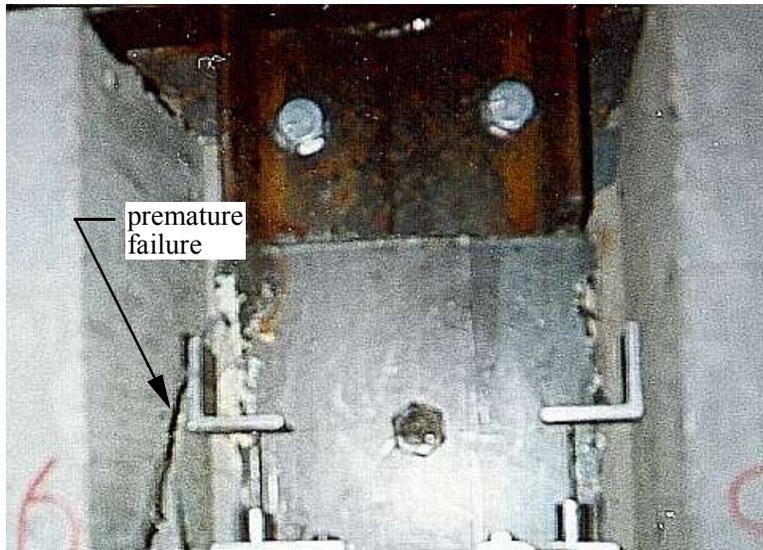
Figure 5.20. Photograph of specimen SH3-6 during testing.
