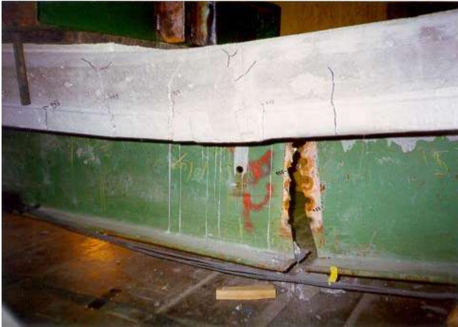
Figure 5.8. Fatigue failure of the steel beam in Specimen 2.
