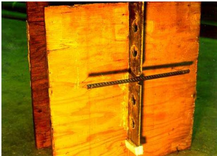
Figure 3.9. Reinforcing bar placed through the shear hole.
