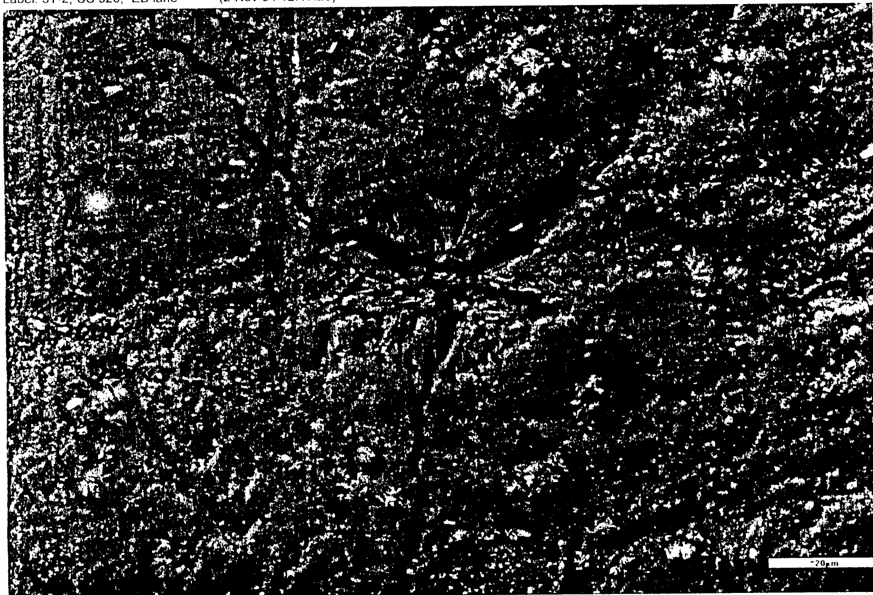
FIGURE 6 A 100X BSE PHOTOMICROGRAPH OF IOWA 20 SHOWING CRACKS RADIATING FROM THE ETTRINGITE FILLED AIR VOIDS
