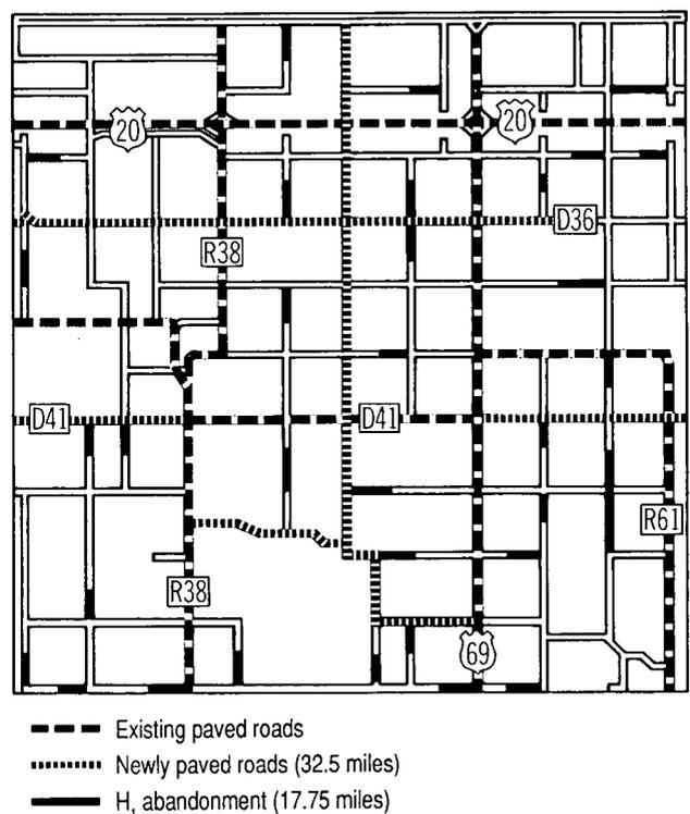
removed from the computerized road network. The network model was rerun to estimate total miles and travel costs for the abandonment solution. Table 3.16 shows the miles of roads that were paved and then abandoned by study area solution.
