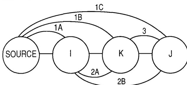
minimized-cost routes between the origin and destination will have been calculated. The number of trips between the original and destination will then be spread evenly over all the routes that are of equal cost. If the route for an origin-destination pair is not found, the computer will select another node to be the source node. This process continues until a minimized-cost route is found for all origin-destination pairs.
