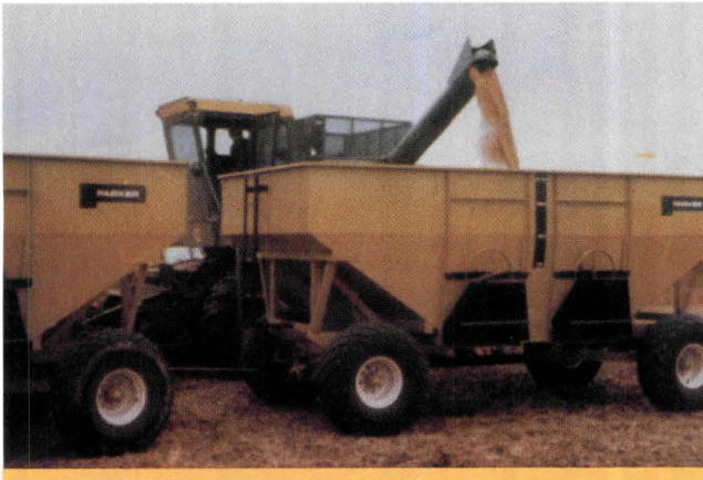
A farm tractor pulling two grain wagons can weigh as much as 36 tons—approaching the federal weight standard and the weight limit in many states. These units, with their shorter length, can concentrate all that weight on a 55-foot bridge at one time.
