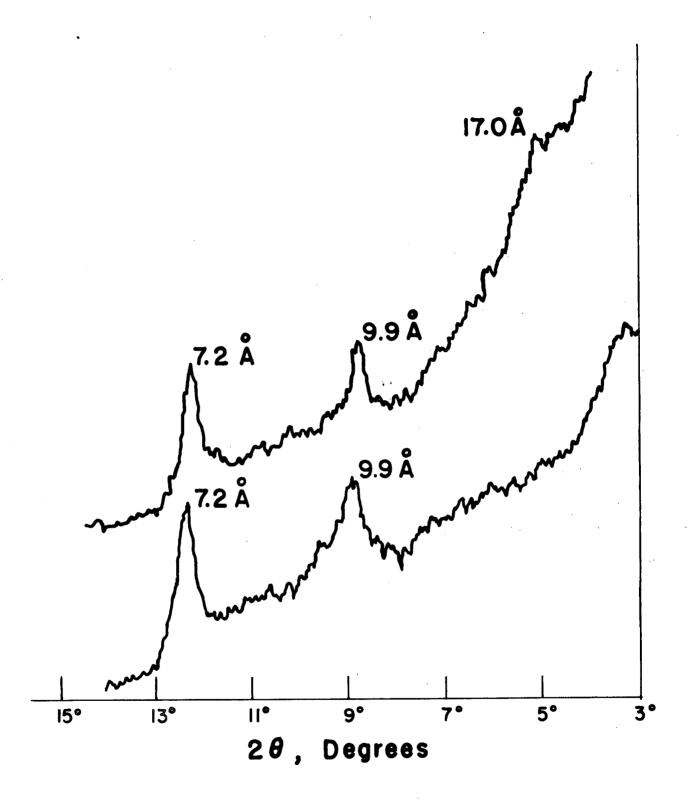
that the montmorillonite is irreversably collapsed after heating to 300°C for a period of one hour or longer (Figure 2). According to Greene-Kelley (2), this irreversibility indicates that the mineral is dioctahedral montmorillonite.
