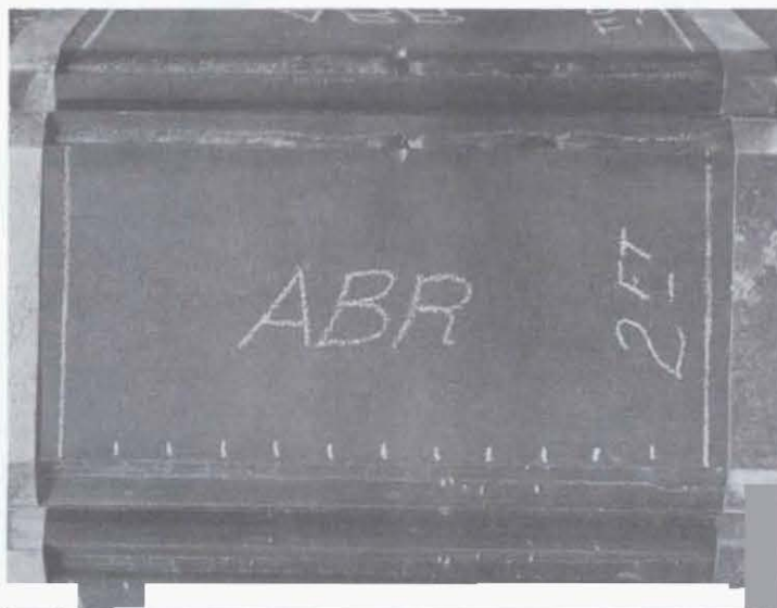
Figure 14. The welds in the Ames beam before testing. Mirror images are at the top and bottom.
