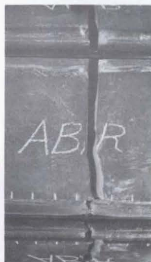
Figure 16. The fatigue crack at end of test.
