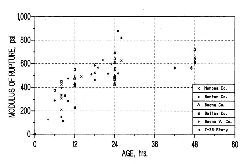
FIGURE 2 BEAM STRENGTHS
