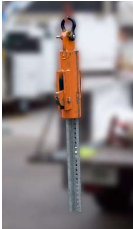
The “post puller” designed by Ron Wolf from Dyersville
