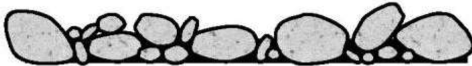
Figure 23. Cross Section of Graded Aggregate in a Thin Maintenance Surface
