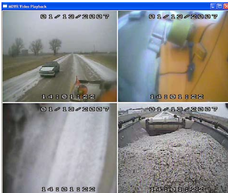
Operators can view all four images being seen by the cameras, either individually or in combination, from a screen in the truck's cab.
