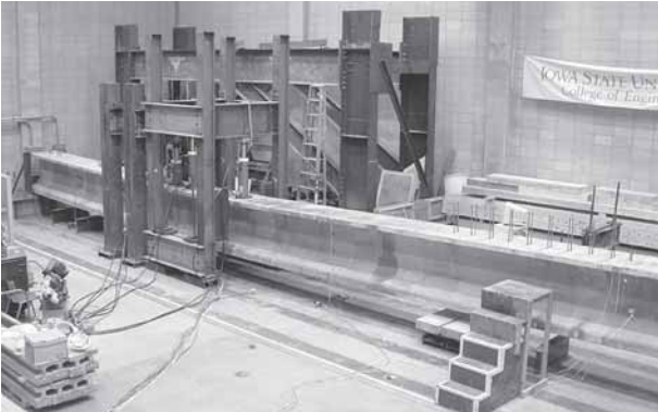
Test three - flexure-shear - Although the beam has a visible sag at the loading frame, cracking was minimal
