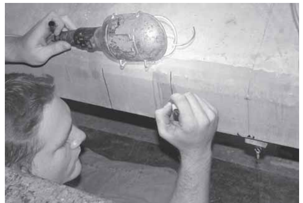
Test one - flexure. Brian Degen, ISU graduate student and former Iowa DOT coop student, marks cracks in the test beam
