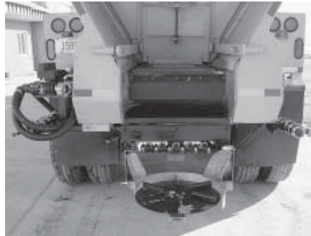
The rear of this Flow Boy trailer has been outfitted with experimental dispersement equipment.
