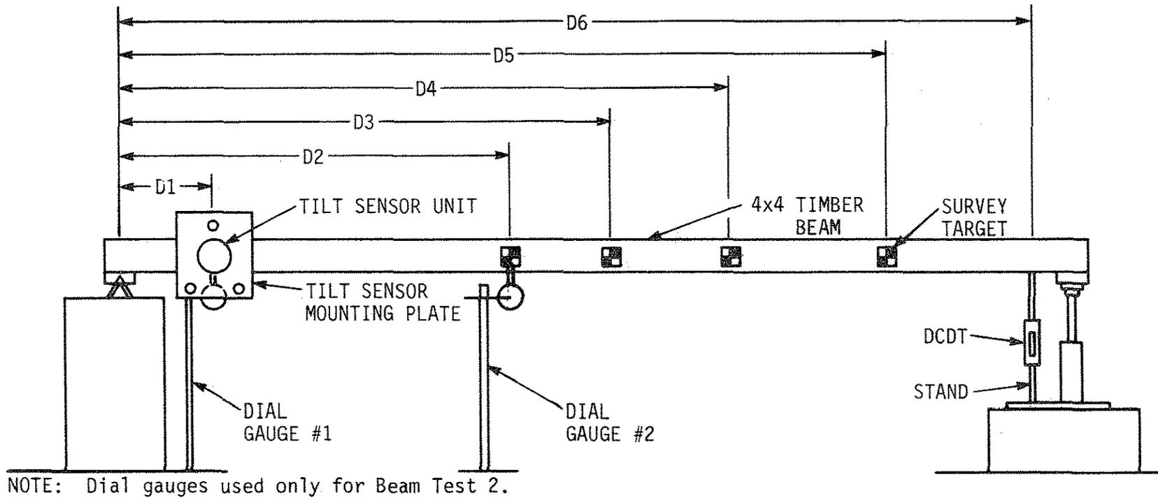
Fig. 18. Instrumentation setup and location for Beam Tests 1 and 2.
