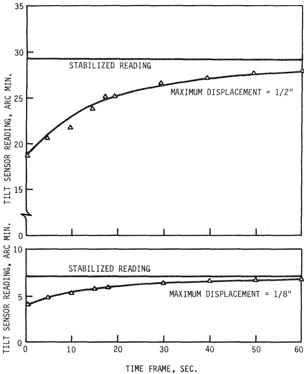
Fig. 26. Plot of response data for the tilt sensor.
