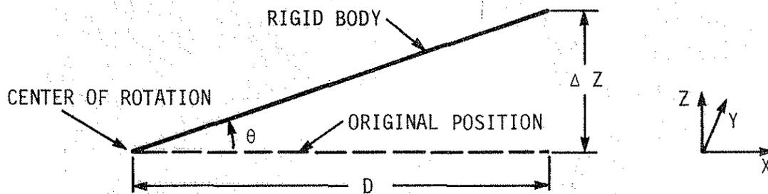
Fig. 4. Description of rigid body rotation for calculating deflections from tilt sensor data.
