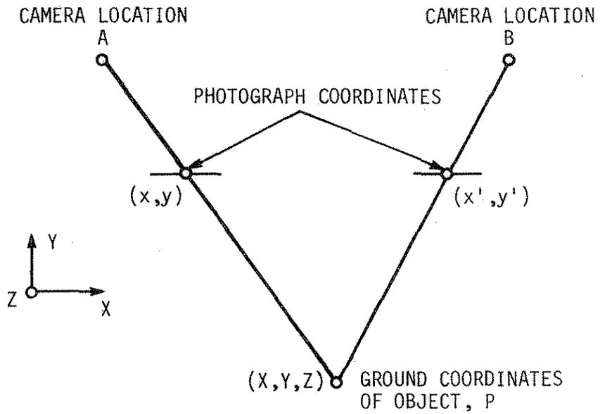
Fig. 9. Plan view of a photogrammetric intersection.
