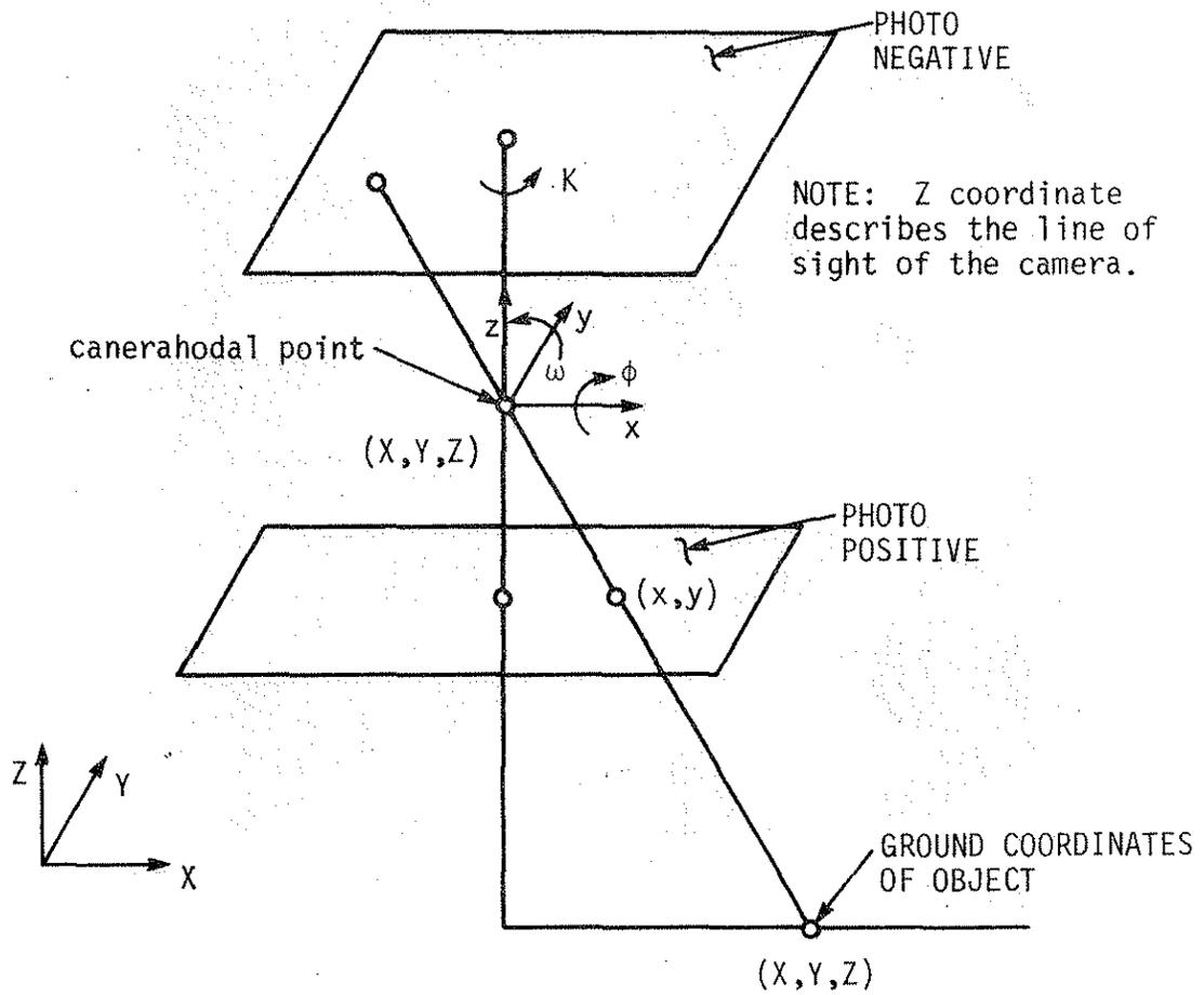
Fig. 8. Photogrammetric resection describing reduction of data for measurements from a photograph.
