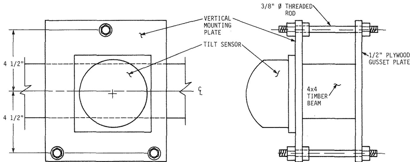
Fig. 19. Details and dimensions of the vertical mounting plate attachment to the beam member.
