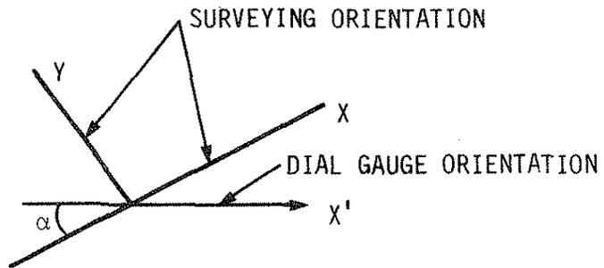
Fig. B.1. Axes' orientation for surveying calculations and movement's orientation as measured by dial gauges.
