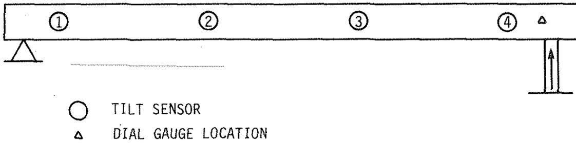
Fig. 25. Location of instrumentation for Beam Test 3.
