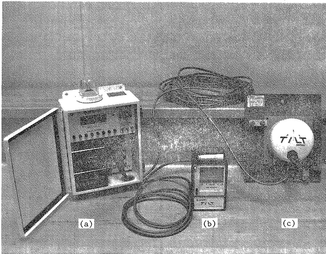
Fig. 2. Tilt sensing equipment: (a) power source, (b) recorder, and (c) tilt sensor and mounting plate.
