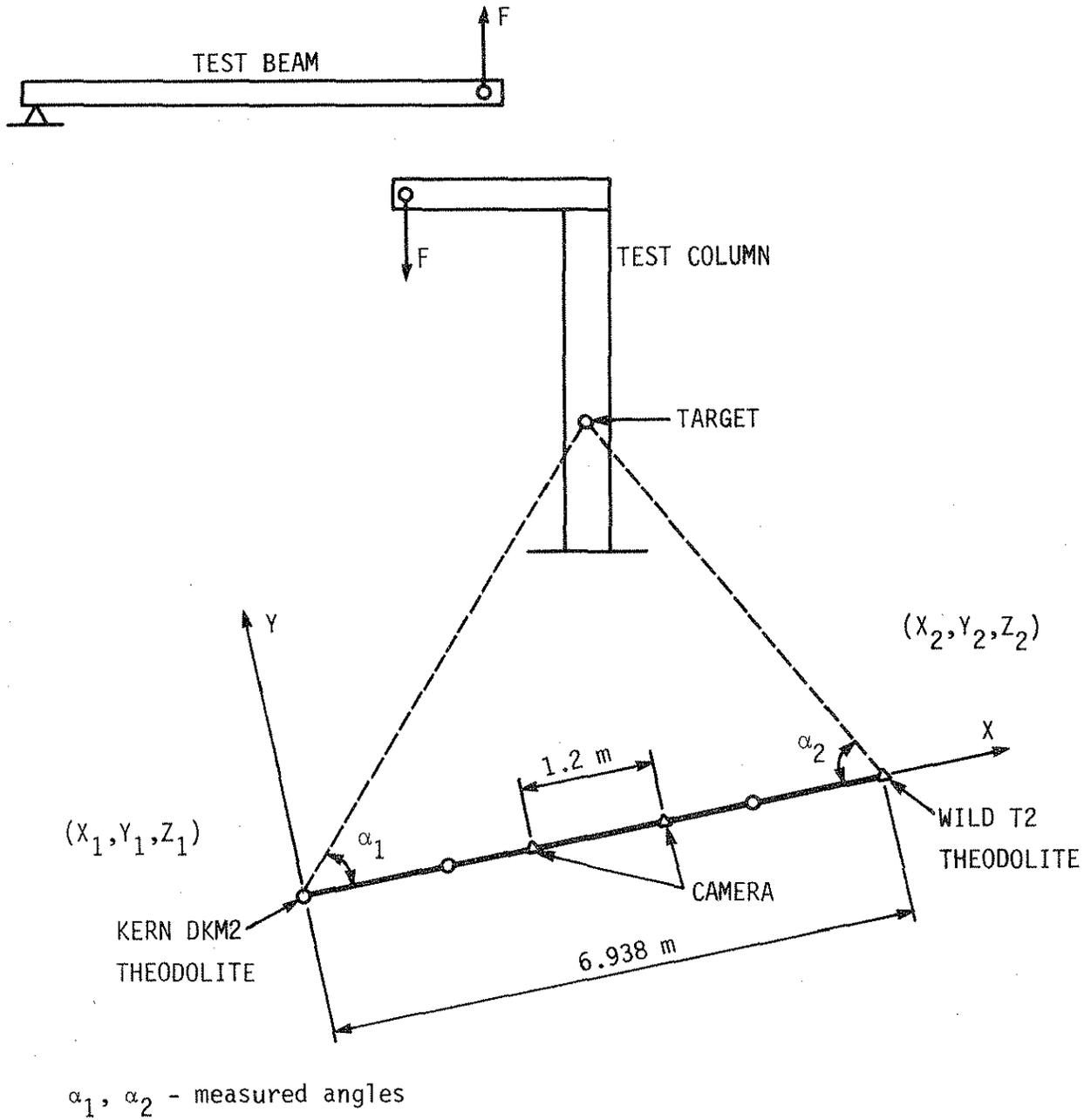
Fig. 16. Baseline and test setup for photogrammetric and surveying methods.
