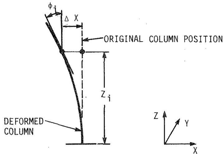
Fig. 5. Description of member curvature for calculating deflection from tilt sensor data.
