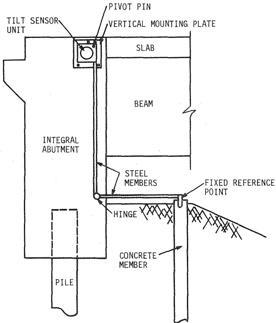
Fig. A.2. Tilt sensor arrangement for monitoring abutment translation (alternative 1).
