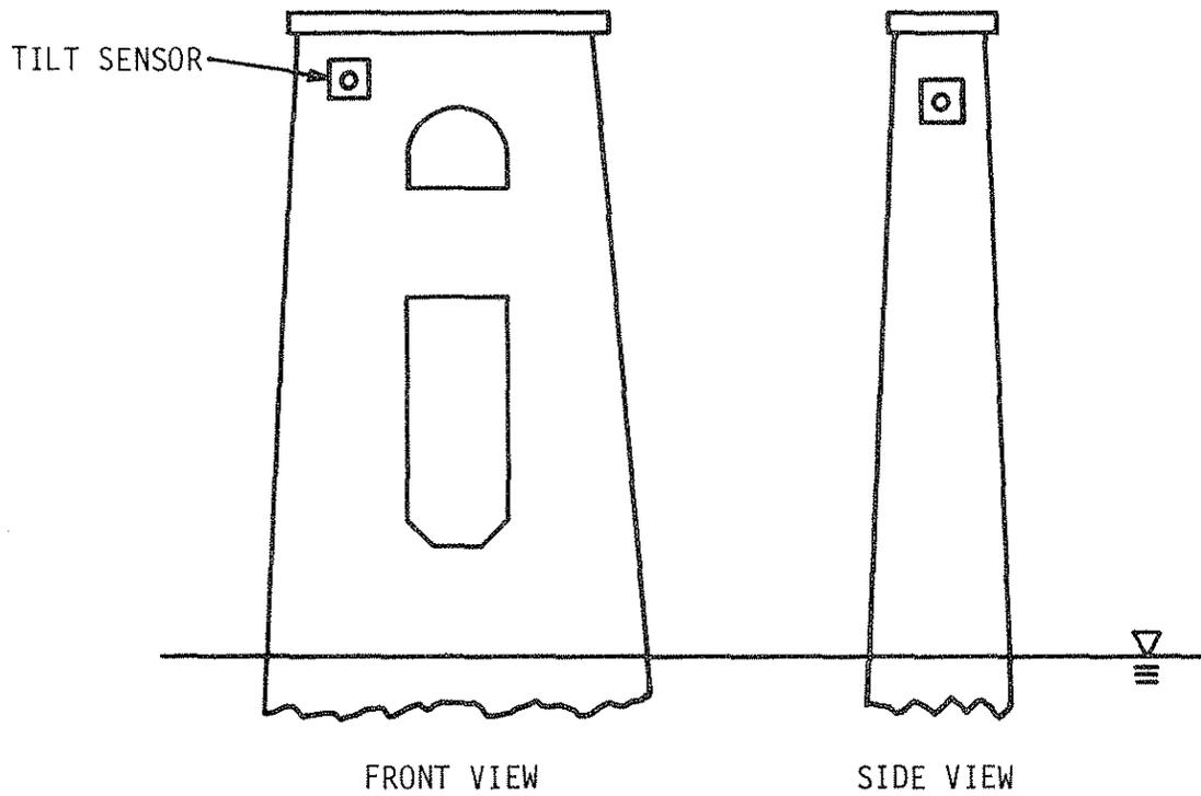
Fig. A.1. Tilt sensor arrangement for monitoring pier movement.
