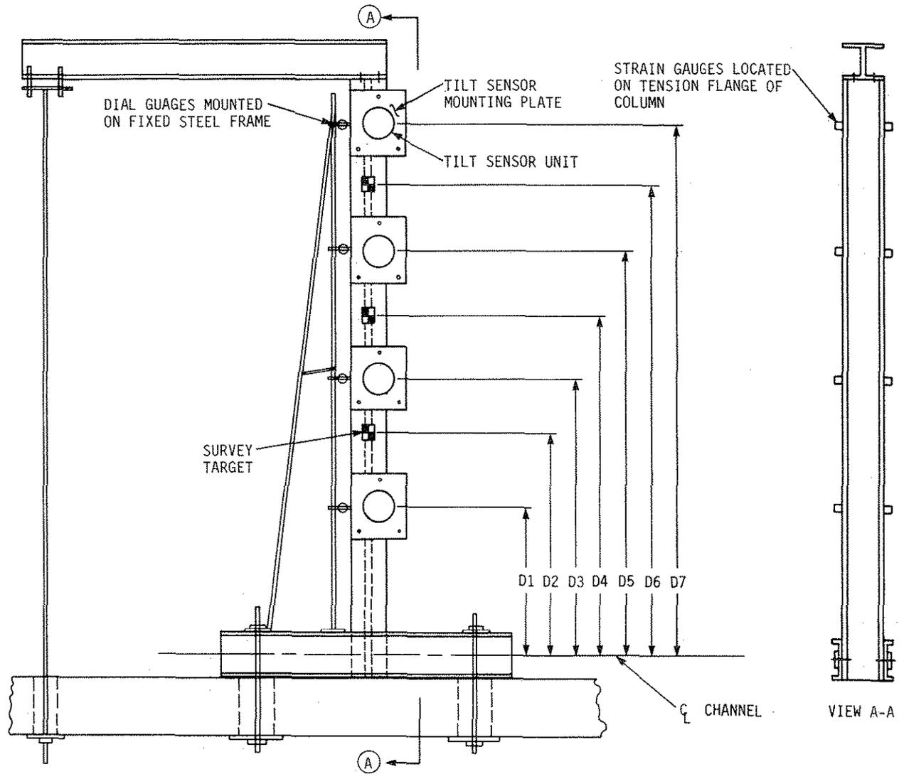
Fig. 14. Test setup and instrumentation for Column Tests 1 and 2.
