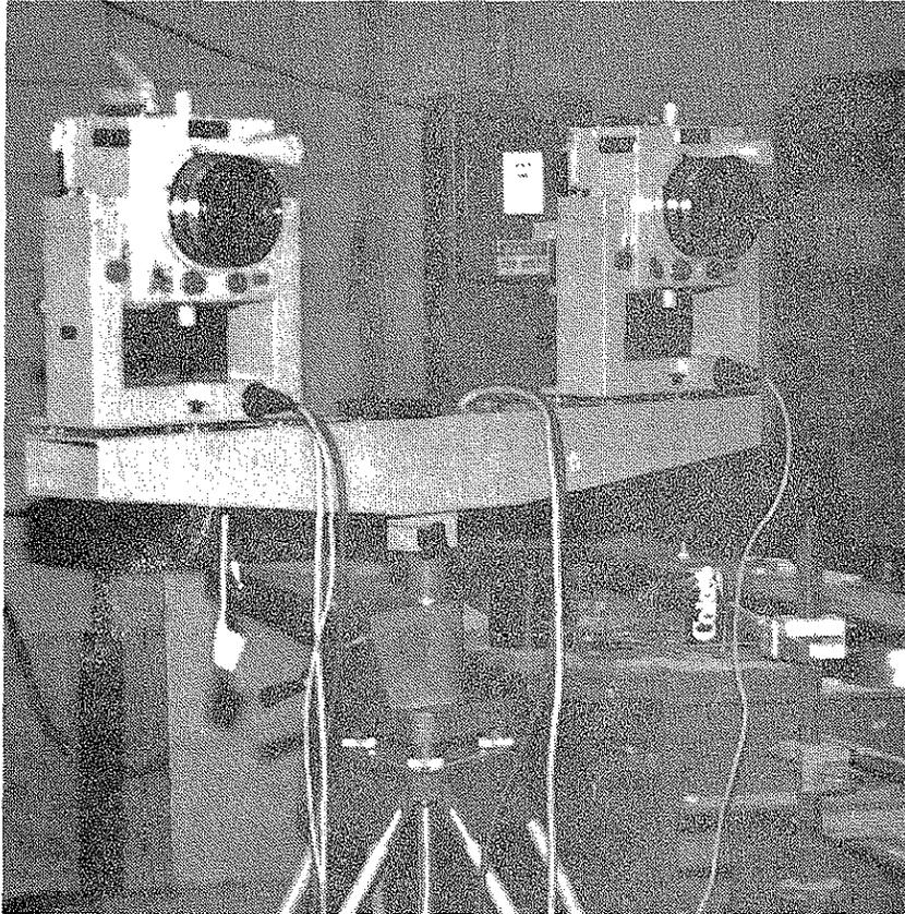
Fig. 7. Zeiss stereometric camera on a tripod.
