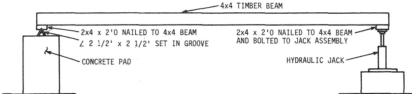
Fig. 12. Member details for Beam Tests 1, 2, and 3.
