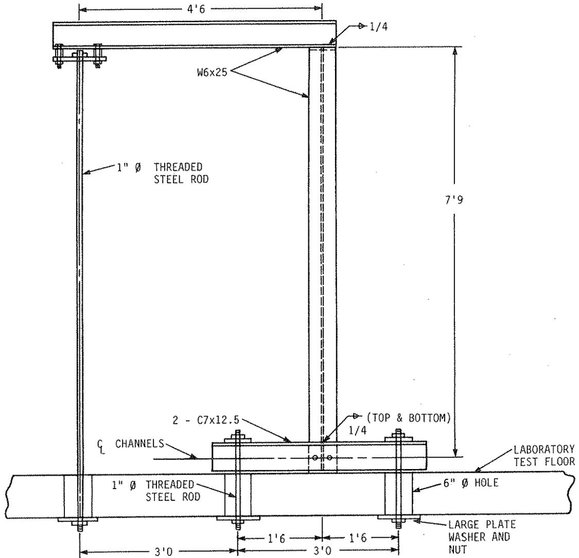
Fig. 11. Frame details for Column Tests 1 and 2.
