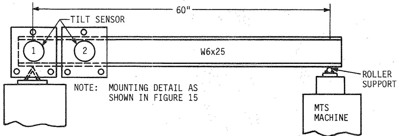
Fig. 21. Test setup for Beam Test 4.
