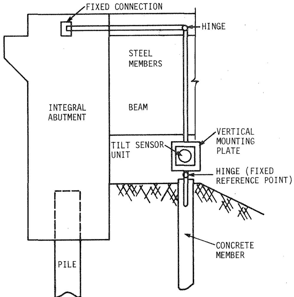
Fig. A.3. Tilt sensor arrangement for monitoring abutment translation (alternative 2).
