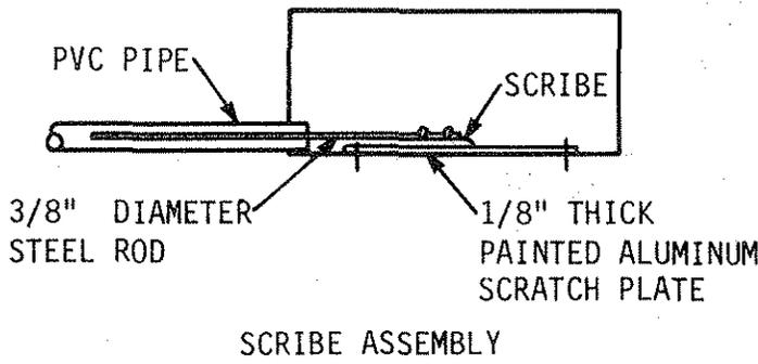
Fig. 1. Detail of assembly used in California study [5] to measure longitudinal movement because of temperature change.
