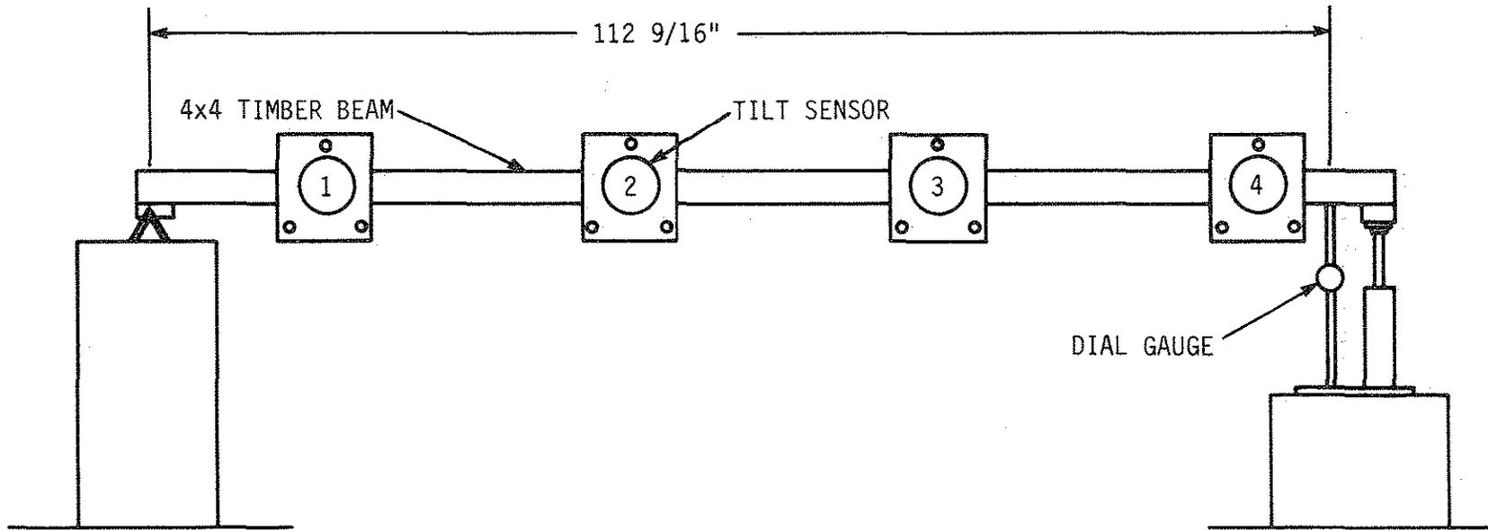
Fig. 20. Test setup for Beam Test 3.
