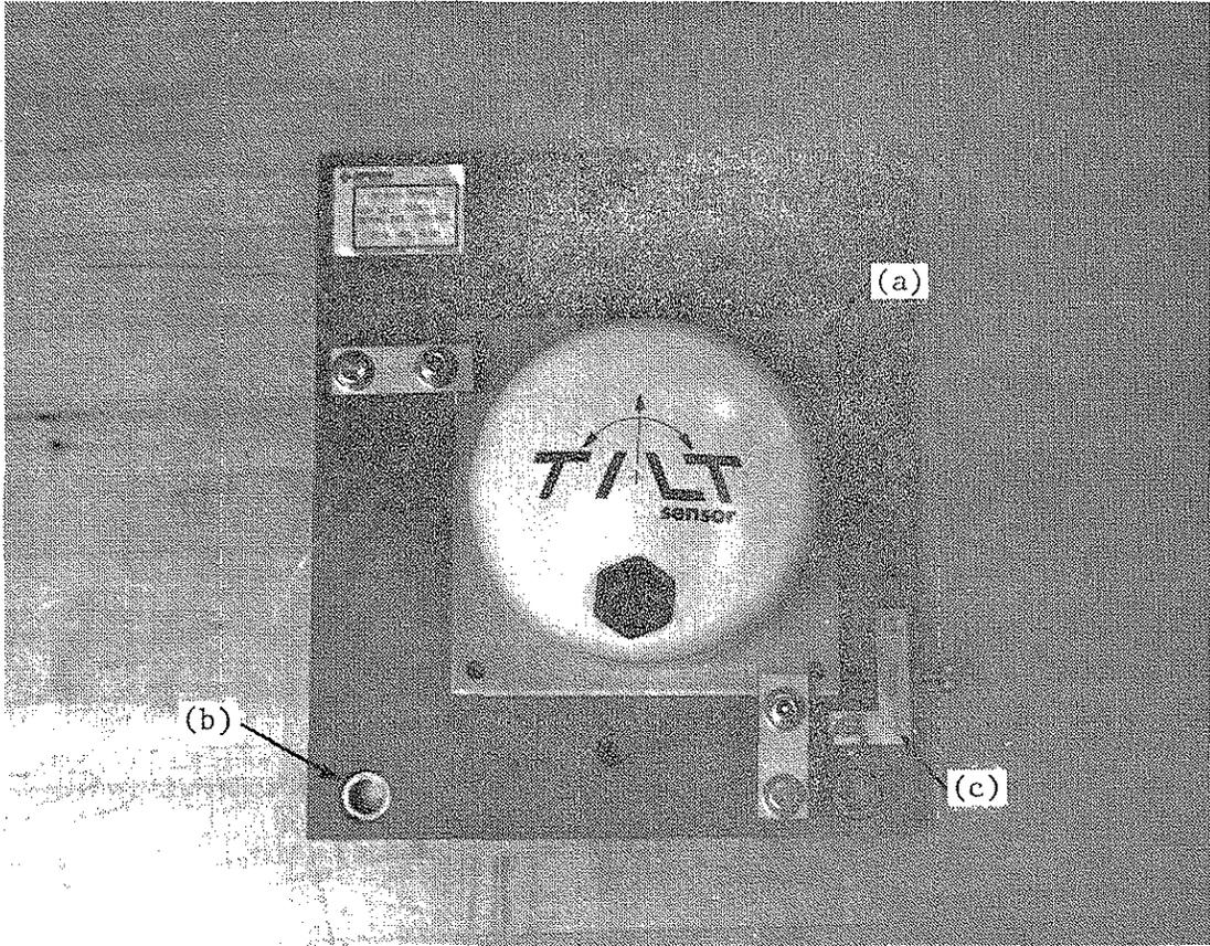
Fig. 3. Details of tilt sensor mounting to the plate: (a) pivot hole, (b) brass mounting pad, and (c) alignment mechanism.
