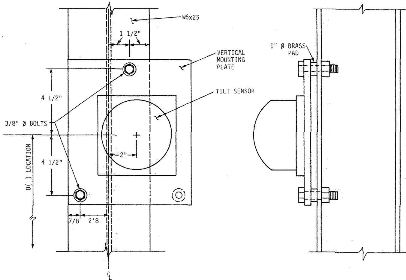
Fig. 15. Details and dimensions of the vertical mounting plate attachment to the column.
