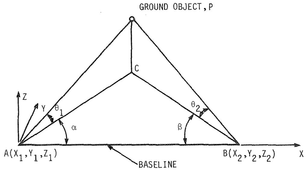
Fig. 10. Three-dimensional view illustrating the concept for making deflection calculations by the surveying method.
