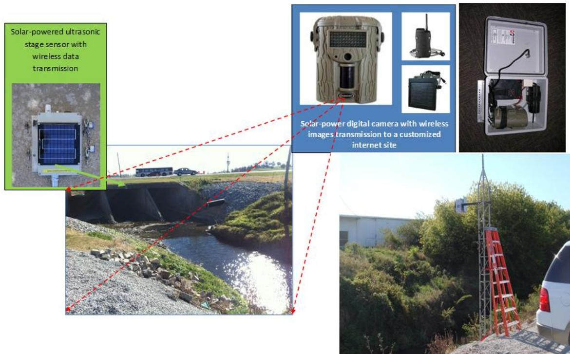
**Figure 15** Real-time webcam deployed at the culvert site under monitoring
