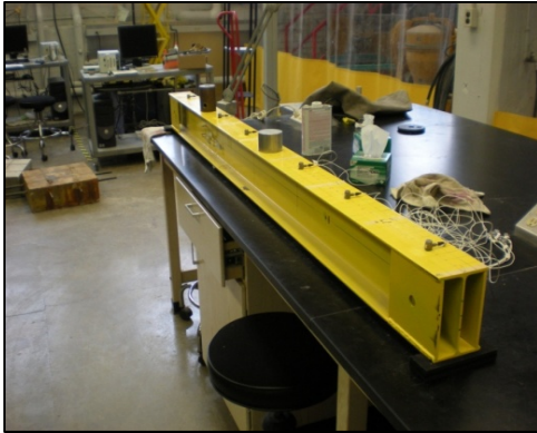
Figure 1 Laboratory I-beam with two damage locations simulated with masses
