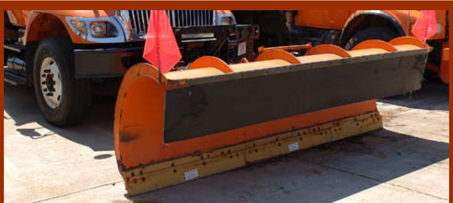
In a stacking-blade set up, a second carbide blade is mounted lower than the original blade to allow all the carbide to be worn down and not damage the moldboard.
