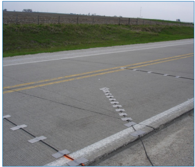
Road tube layout to measure lateral displacement in the field (Z configuration)
