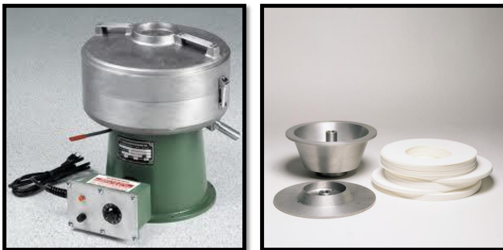
Figure 3.12 First centrifuge with bowl and filter paper
