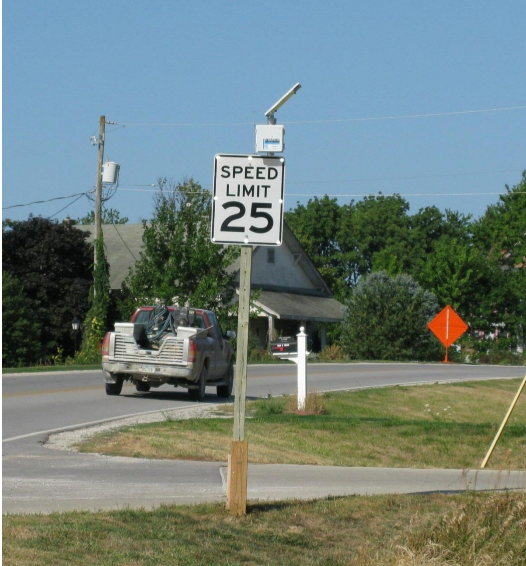
Figure 5-17: Radar-activated LED speed limit sign at east St. Charles community entrance
