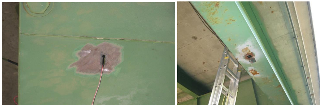
Figure 18. Weldable strain gauge
