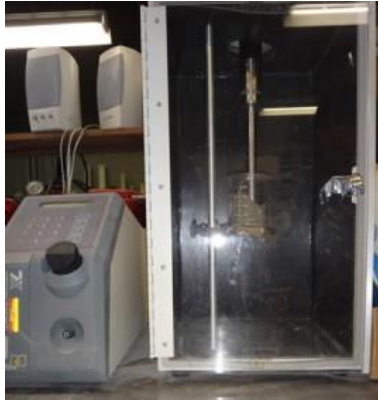
Figure 3.2. Sonicator XL-2020 ultrasonic processor used in mixing process
