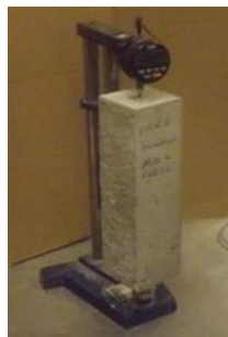
Figure 3.9. Length measurements of concrete specimens
