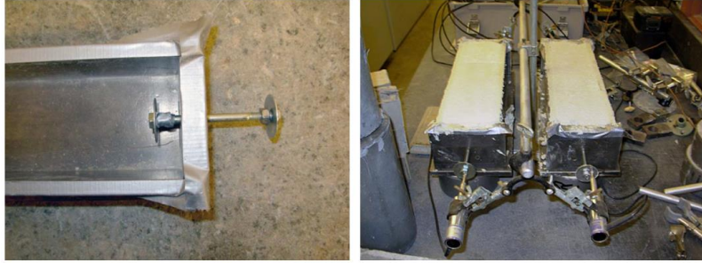
Figure 2.11. Bolt/washer assembly and test setup with LVDTs (Mokarem et al. 2008)
