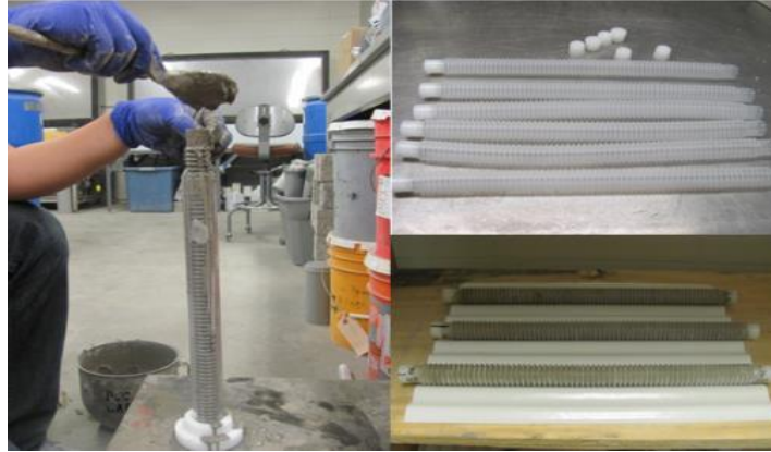
Figure 3.4. Specimen preparations for autogenous shrinkage of mortar
