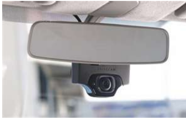
Figure 2. DriveCam Event-Triggered Video Data Recorder
