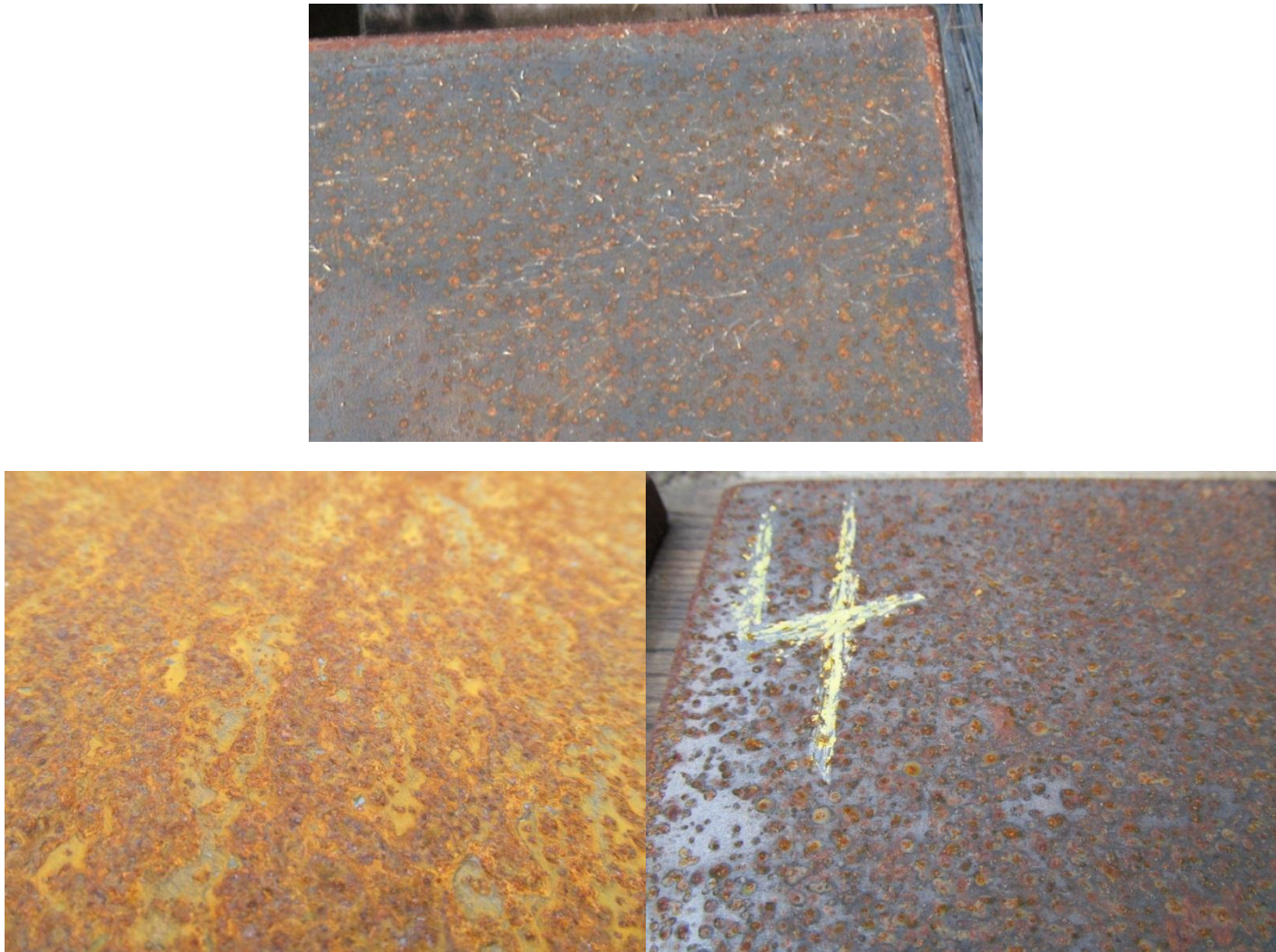
Figure 8. Close-up photos of plate condition before testing (top center), after salt spray (bottom left), and after deionized water spray (bottom right).
