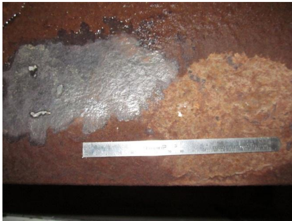
Figure 3. Close-up of wire wheel ground area and adjacent as-is poultice after washing and drying.
