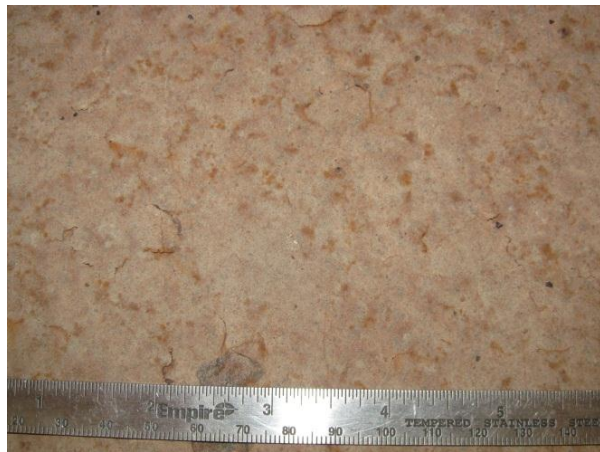
Figure 1. Top of bottom flange poultice prior to washing; Index = 2, chlorides measured = 20 ppm.
