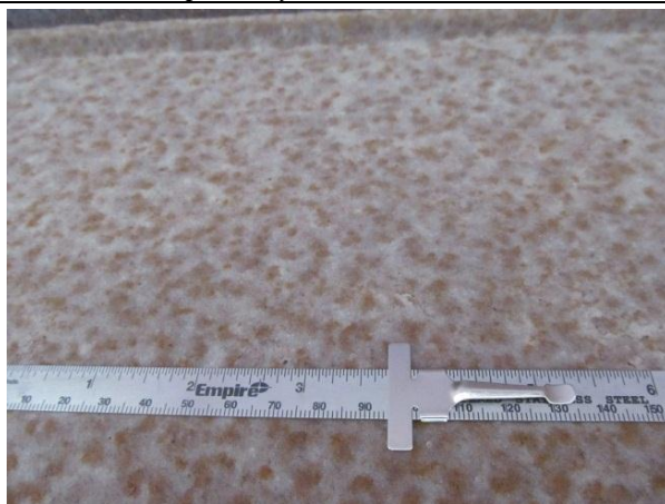
Figure 5. Poulitice on flange before washing.
