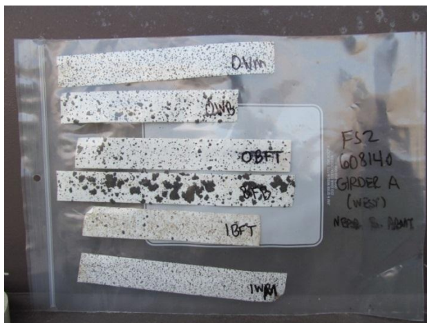
Figure 5. Tape test series taken from west fascia girder adjacent to downspout showing large flakes (Index=2) on bottom of bottom flange.
