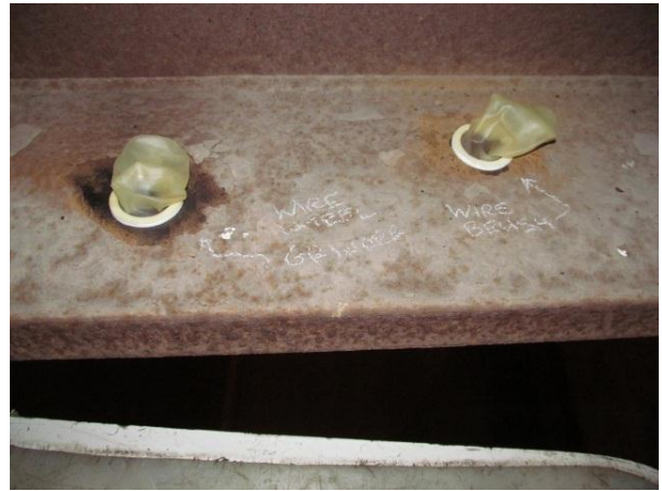
Figure 2. Chloride tests with some leaking on chalky poultice of bottom flange before washing.
