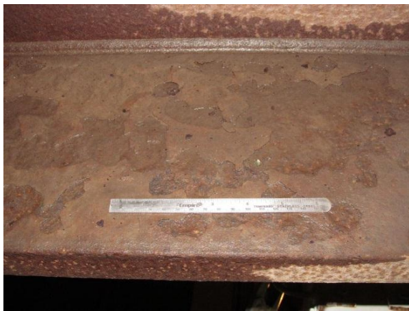
Figure 5. Washing as-is: poultice reduced, but delamination remains.
