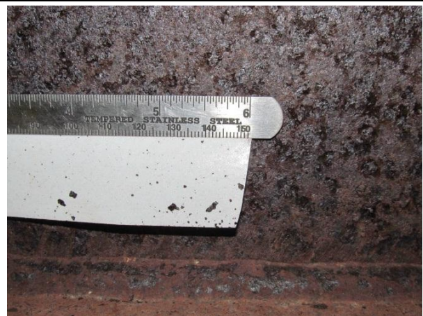
Figure 6. Bottom of web after washing; tape test (sparse, Index = 3) shows improvement in adherence (Index before = 2 with dense coverage).
