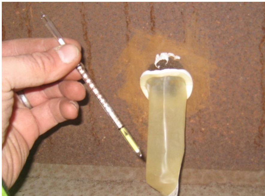
Figure 31. CHLOR*TEST glass tube ready for insertion into sleeve to read results.
