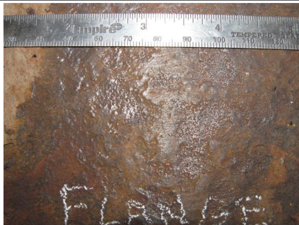
Figure 3. Top of bottom flange ground with wire wheel. Chlorides in ground area before washing = 20 ppm; after washing, 14 ppm extracted by test.
