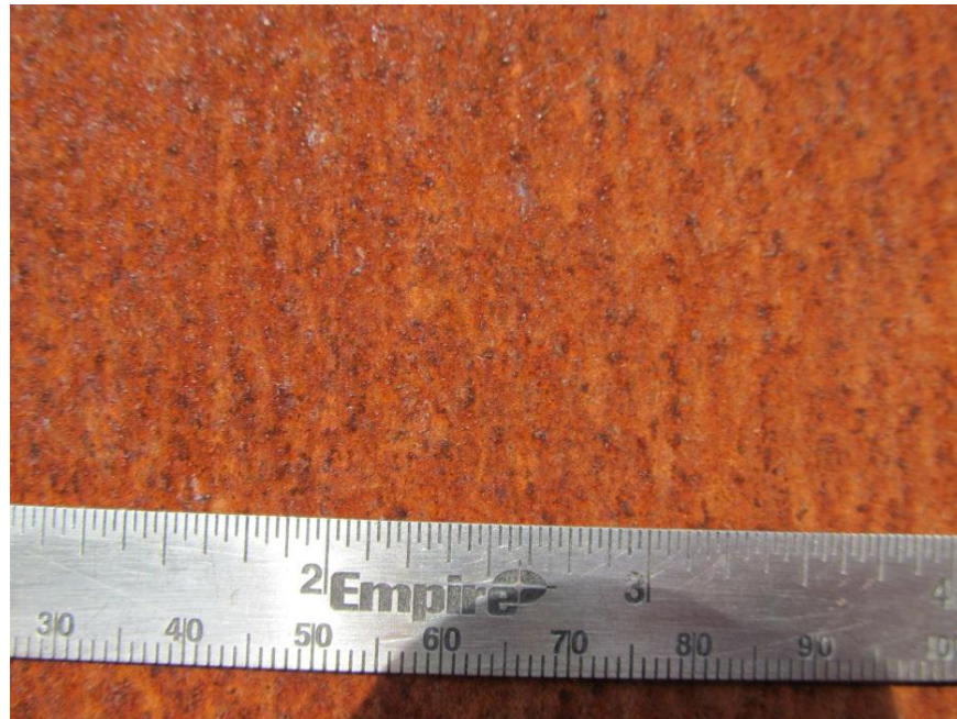
Figure 16. Close-up photo of Category 5 patina taken from Illinois pedestrian bridge truss. Only isolated regions of Category 5 patina, likely due to mill scale, were observed on Iowa bridges.
