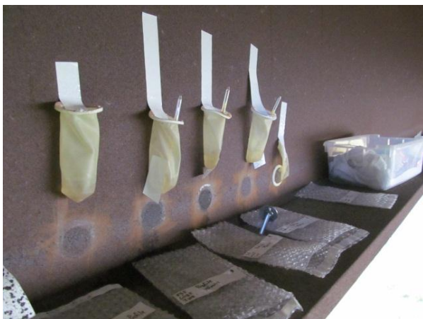
Figure 5. Chloride test time vs. extraction efficiency profile taken on bottom of interior web (Index = 3).
