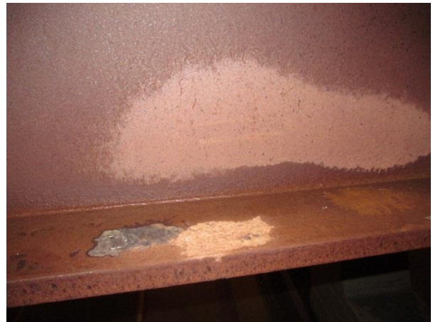
Figure 4. Test area after washing and partial drying: wire wheel area on left, wire brush area on far right.
