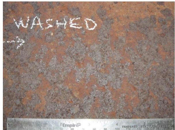
Figure 2. Top of bottom flange after washing; some of poultice remains, Index = 2, chlorides = 10 ppm.
