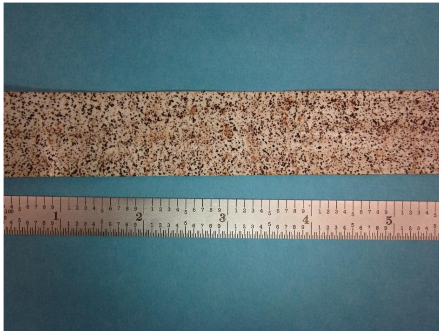
Figure 23. Category 5 tape test sample; note fine reddish rust phase particulates interspersed with more typical dark brown patina flakes.
