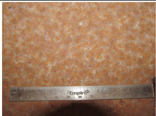
Figure 6. Flange poulitice partially reduced by washing.
