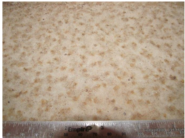
Figure 4. Heavy flange chalking with only minor flaking (Index = 3).
