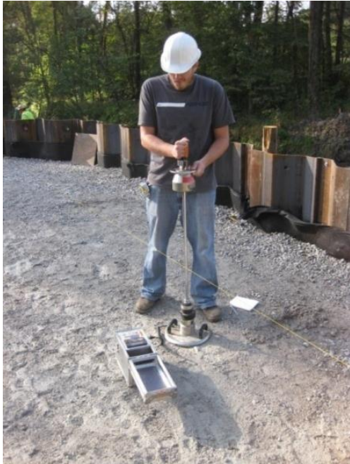
a.) Testing on abutment backfill at base of spread footing
