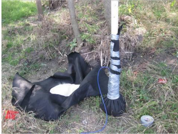
Figure 5-25. Piezometer assembly for water table monitoring
