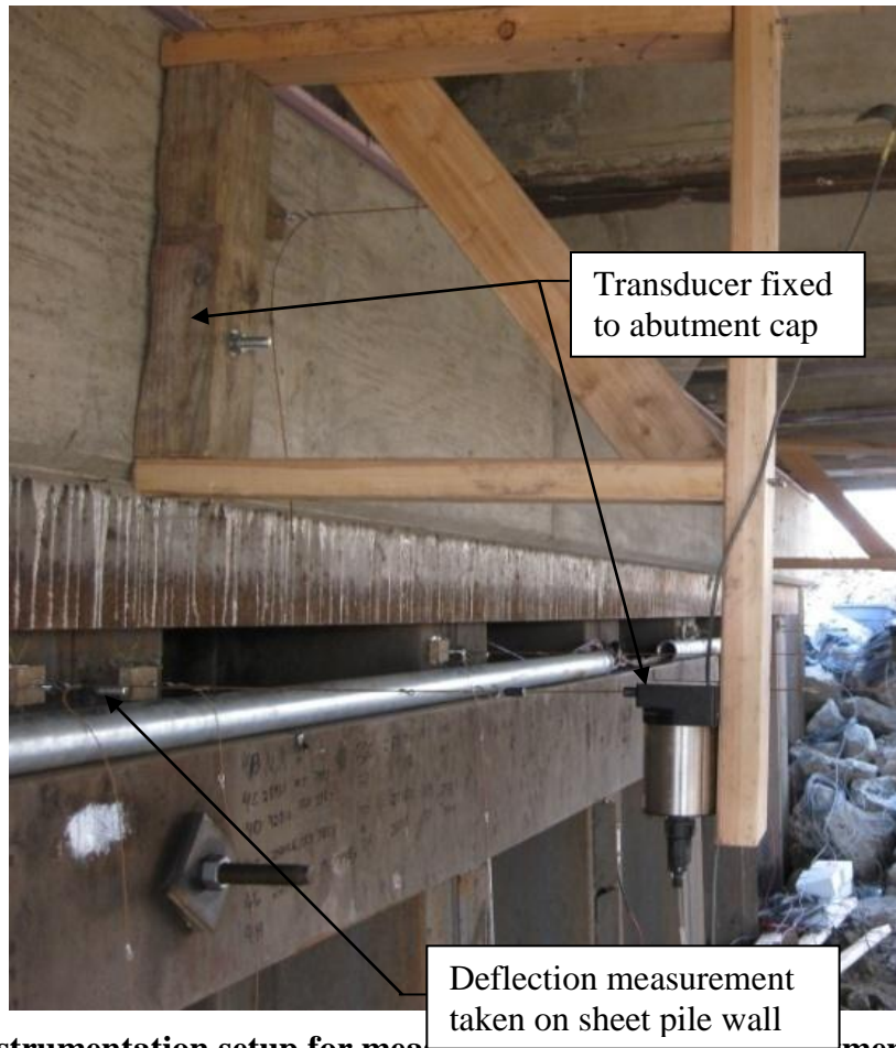
Figure 5-39. Instrumentation setup for measuring displacement of abutment cap relative to sheet pile wall (Disp 003)
