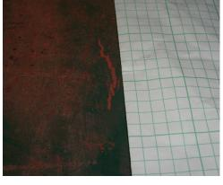
b. Top Web-Plate Cracking
