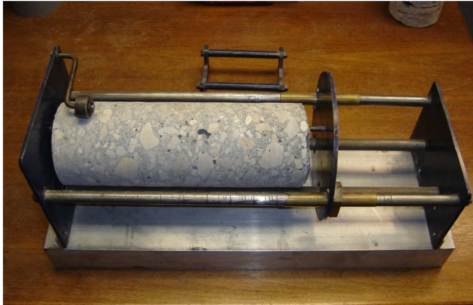
Figure 9 Iowa Department of Transportation nine point core measurement apparatus.
