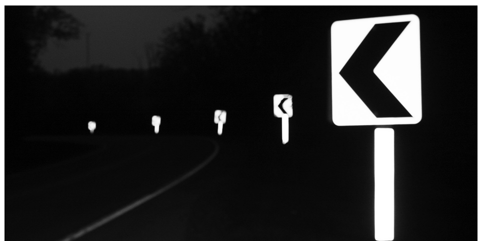
Retroreflective signs on US 52 in Iowa help drivers anticipate an upcoming curve at night
