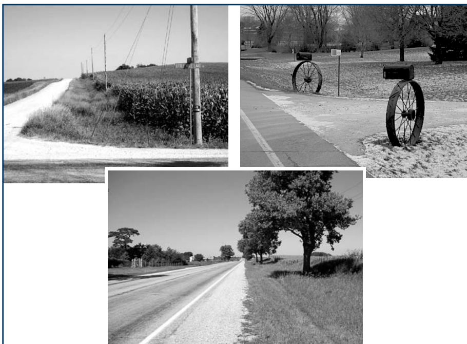
Examples of hazards in clear zone that can affect crash severity (Photos courtesy of Jack Latterell)
