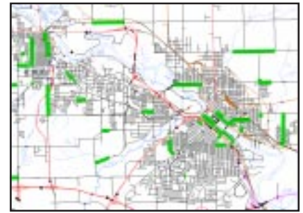
The pavement management GIS database can be queried and the results displayed graphically. For example, data about roadways with poor ride quality (displayed by green lines, above right) and data about roadway cracking (pink lines, above left) can be overlaid to show where roadway cracking may be affecting ride quality (circled areas, below).
