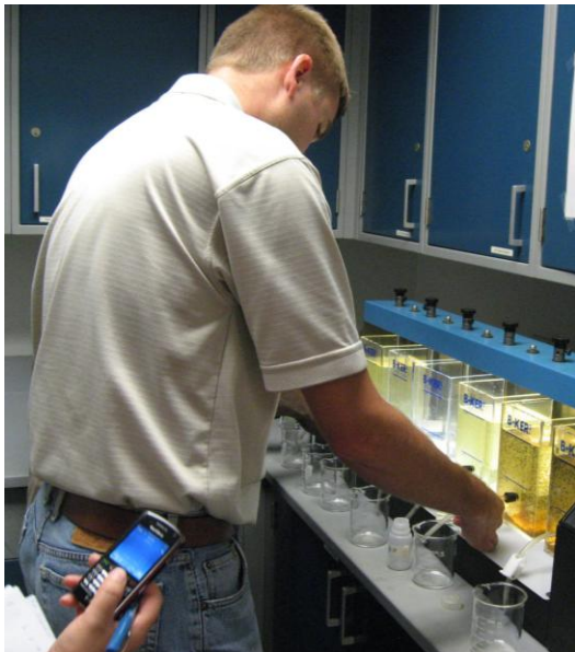
Performance-based Training, Round 2 (Session #3 in 2010) – Jar testing different coagulant dosages to optimize the coagulation and flocculation processes
