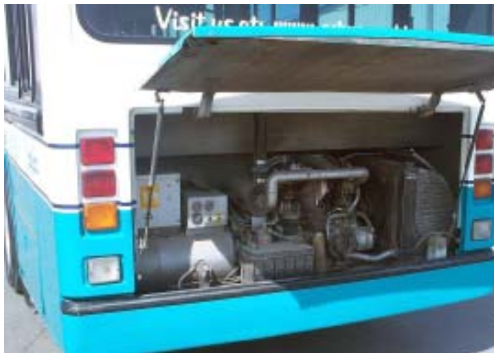
(Top) This very average looking bus is one of the nine most environmentally friendly buses anywhere in Iowa. Its batteries power an electric engine that permits service to be provided with dramatically reduced overall emissions. (Above) Environmental awareness in Cedar Rapids has resulted in this bus showcasing its unique engine compartment. Shown here are some of the hybrid diesel electric drive train components being tested by Five Seasons Transportation and Parking.
