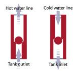
If anti-convection valves or heat traps for both the cold-water inlet and the hot water outlet are not included with your new water heater, make sure the installer adds them.
