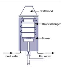
A tankless water heater can be a sensible choice in a home occupied by just one or two people—or a family with a schedule that doesn't require multiple hot water uses at the same time.
