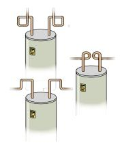
Heat traps fabricated from copper plumbing pipe can help prevent heat loss from a storage-type water heater.
