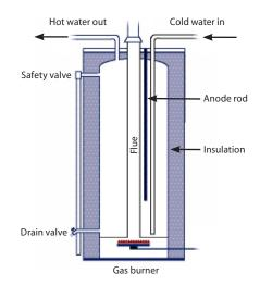
In a natural gas or propane storage tank water heater, the burner sits below the water tank-but within the insulated shell of the unit. In most cases, recovery time for a gas water heater will be shorter than that of an electric unit.
