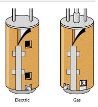
Wrapping an **insulation blanket** around the tank of your existing gas or electric water heater can save you money on water-heating bills. The insulation blanket will reduce standby heat loss—heat lost through the wall of the tank—by 25% to 45%, and you'll likely recover the cost of the blanket through reduced water-heating bills within a year.
