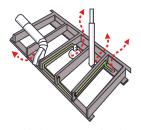
Recessed lights, wiring, plumbing and other openings in insulated ceilings and walls can result in a tremendous amount of heat loss.
