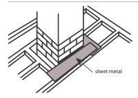
Heat can escape around the chimney if it isn't properly sealed with sheet metal and the appropriate caulk.
