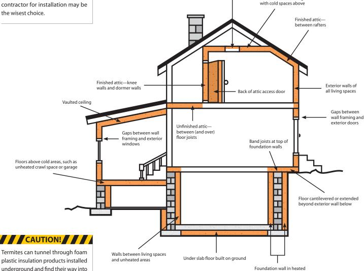
Termites can tunnel through foam plastic insulation products installed underground and find their way into your home's structure. If termites are a problem in your area, talk with an insulation professional about using termite-resistant products and preventing termite infestations by other means.
