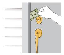
Check for air leaks in weather stripping around windows and exterior doors by closing them on a dollar bill or a strip of paper in several locations around their perimeters. If you easily can remove the bill (or it falls out), the weather stripping needs to be repaired or replaced. Also perform a visual check of every weather strip, looking for cracked, deformed or missing sections.
