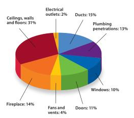
Air infiltrates into your home through every hole, nook and cranny. About onethird of this air infiltrates through the openings in your ceilings, walls and floors.
