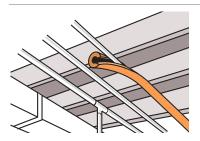
Use foam insulation on hot water pipes in your basement or crawl space. The water will stay warmer in the pipes, cutting the time you need to wait for hot water for sinks, bathtubs or showers.
