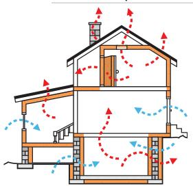
Plugging air leaks after a careful inspection of your home's structure—both inside and outside—can yield a significant reduction on your monthly heating and cooling bill. In this illustration, blue arrows indicate outside air infiltration and red arrows show where conditioned (heated or cooled) air can escape.
