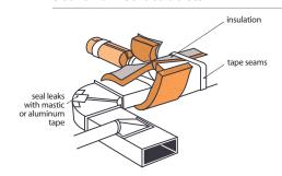
Tighten and seal leaky ducts before insulating with foil- or paper-faced batts made especially for ducts.
