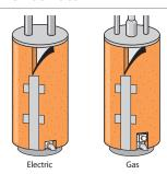
Giving your older water heater a blanket to lower your water-heating bills is an easy, do-it-yourself job. Be sure to follow the insulation manufacturer's installation instructions—the process differs for electric and gas water heaters. Note that new water heaters have adequate insulation, so their manufacturers recommend not adding an insulating blanket.
