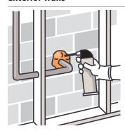
Expanding foam sealant works well for sealing gaps more than 1/4-inch wide.
