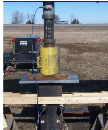
(d) Placed load cell and jack between test pile and beam
