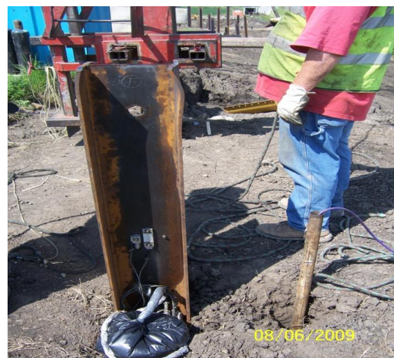
(d) Measuring pore water pressure and lateral earth pressure
