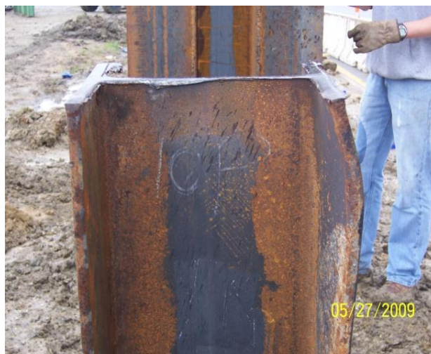
Figure 4.16. Minimal buckling on flanges at pile head
