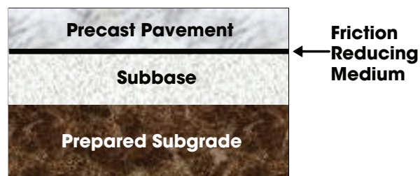
Figure 4-1. Precast pavement system cross-section
