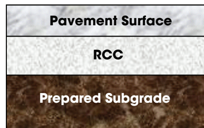
Figure 5-3. Pavement cross-section with RCC base
