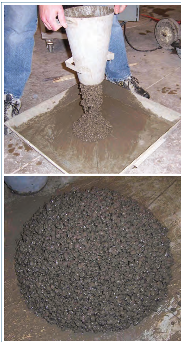
Figure 3-6. Fresh pervious concrete
