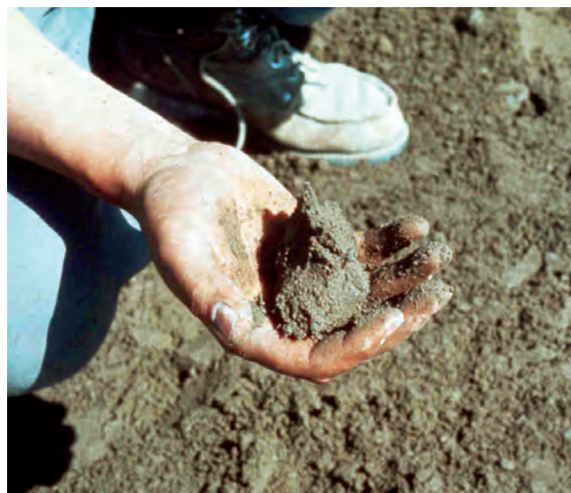
Figure 5-6. RCC material looks drier than conventional concrete
