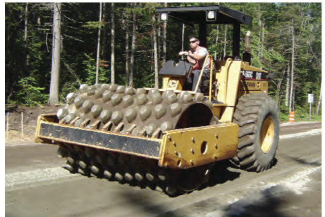
Figure 8-4. Sheepsfoot roller used for compaction
