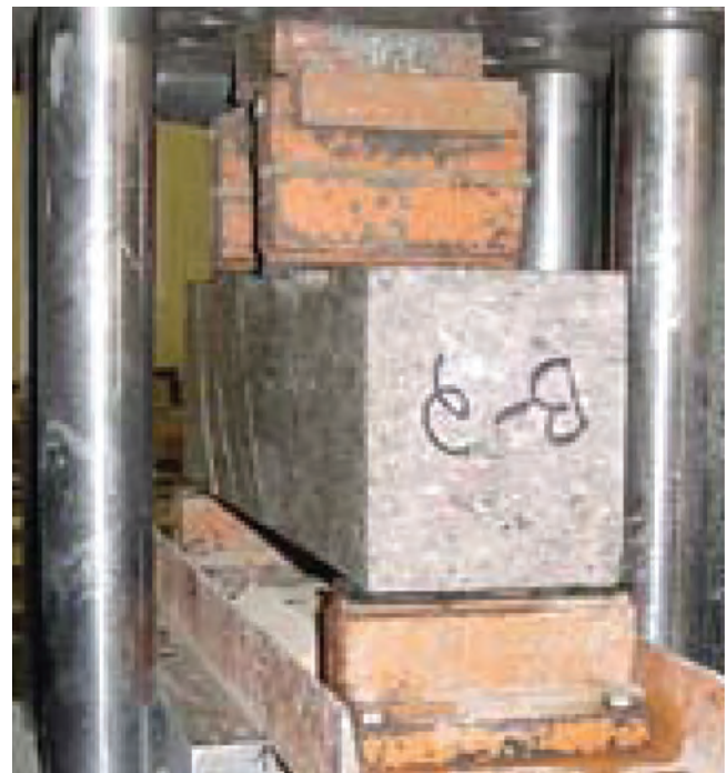
Figure 5-7. Flexural beam testing
