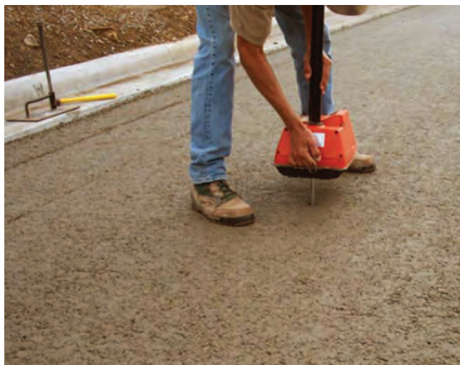
Figure 5-15. RCC in-place density measurement
