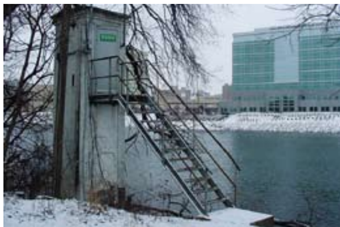
A typical USGS streamflow-gauge with satellite telemetry
