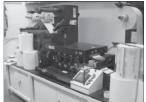
Above: License plates are produced using a digital system of thermal transfer printing.
