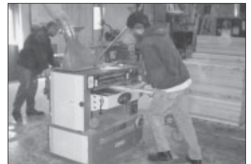
Inmate Gray (left) & Lead Inmate Klindt (right) mill rungs for loft bed ends using the new spiral cut planer.
