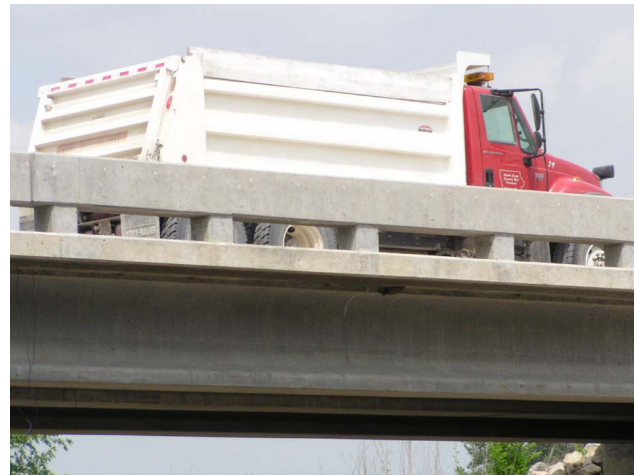
Vehicle used for second live load test on Wapello County UHPC bridge
