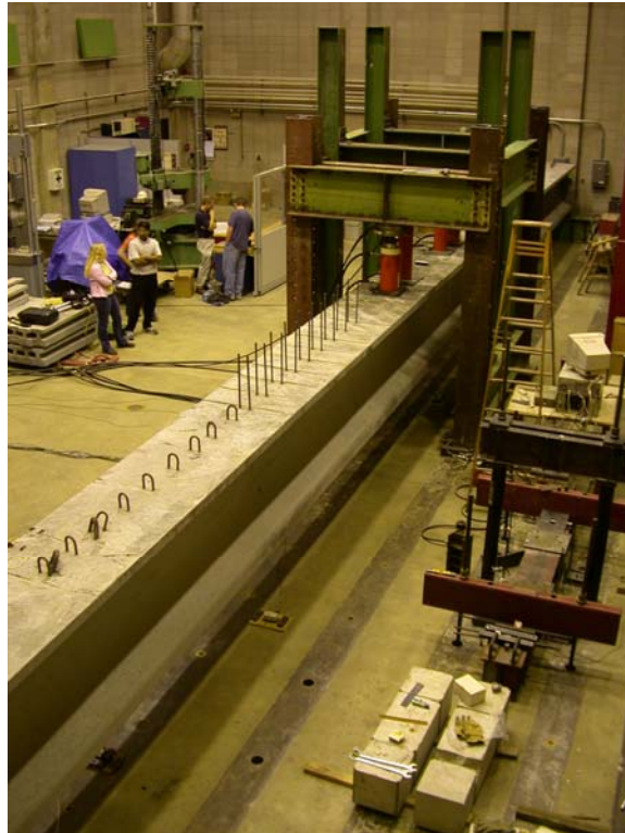
Figure 4.4. Large-scale flexure test setup photograph.
