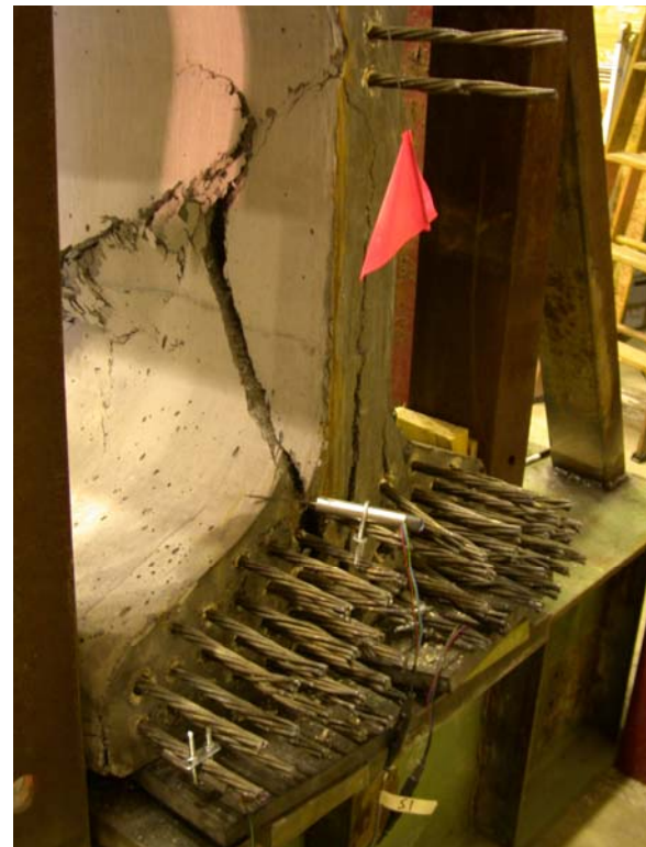
Figure 6.8. Vertical crack in web at west end of large-scale shear test beam after failure.
