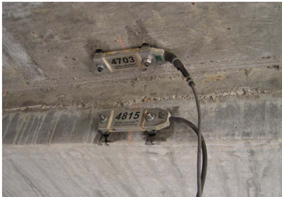
Figure 4.25. BDI strain transducers attached to concrete.
