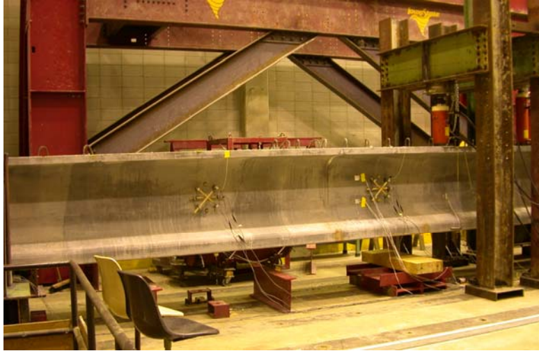
Figure 4.13. Large-scale flexure-shear test setup photograph.
