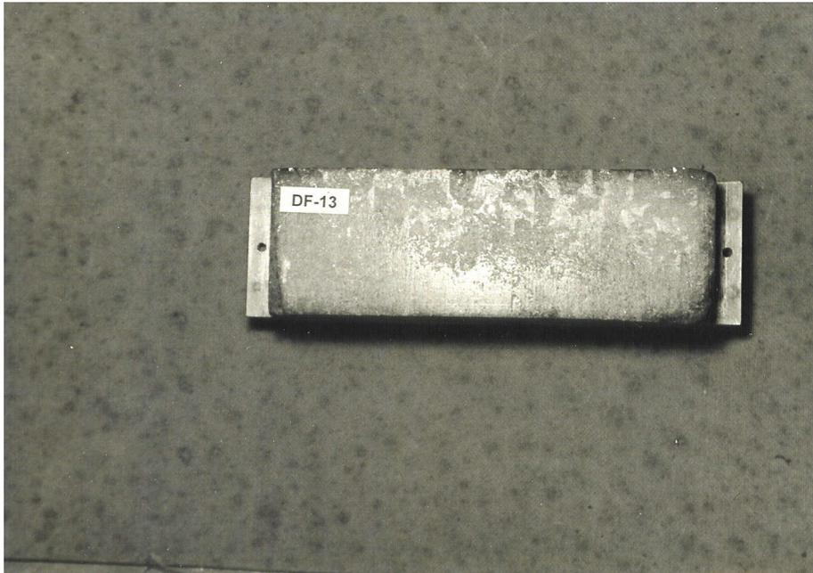
Figure 2.1: Typical Concrete Test Specimen
