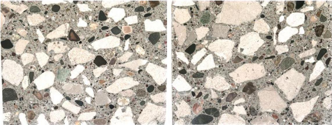
**Figure 8 – Woodbine optical images (salt) - middle (l), edge (r)**
