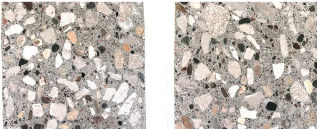
**Figure 4 – Rockford optical images (salt) - middle (l), edge (r)**
