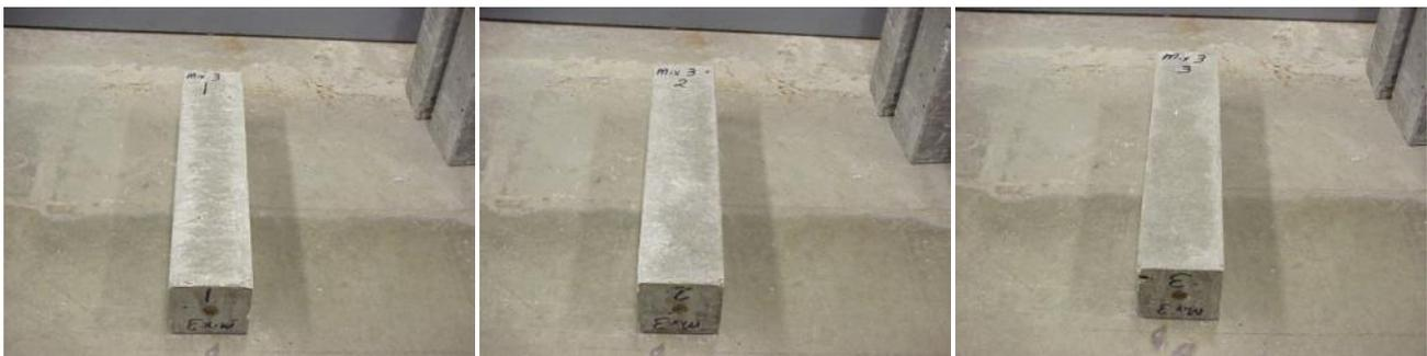
Figure 23 – Army Post Road freeze thaw beams (salt)
