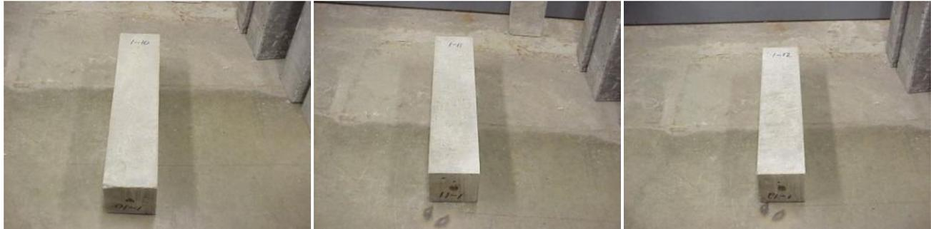
Figure 20 – Ames South freeze thaw beams (no salt)
