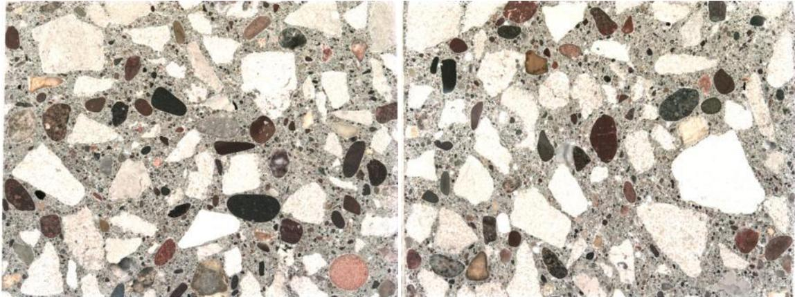
Little deterioration was noted in any of the samples investigated. Salt was concentrated in a rim around a few aggregate particles, but no deterioration was noted. Pyrite, found in some samples, also exhibited little signs of deterioration.
