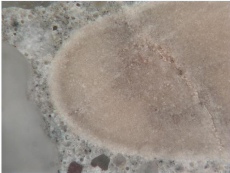
**Figure 12 – Pyrite in Bellevue salt sample**
