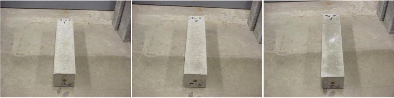
Figure 25 – Harlan freeze thaw beams (salt)
