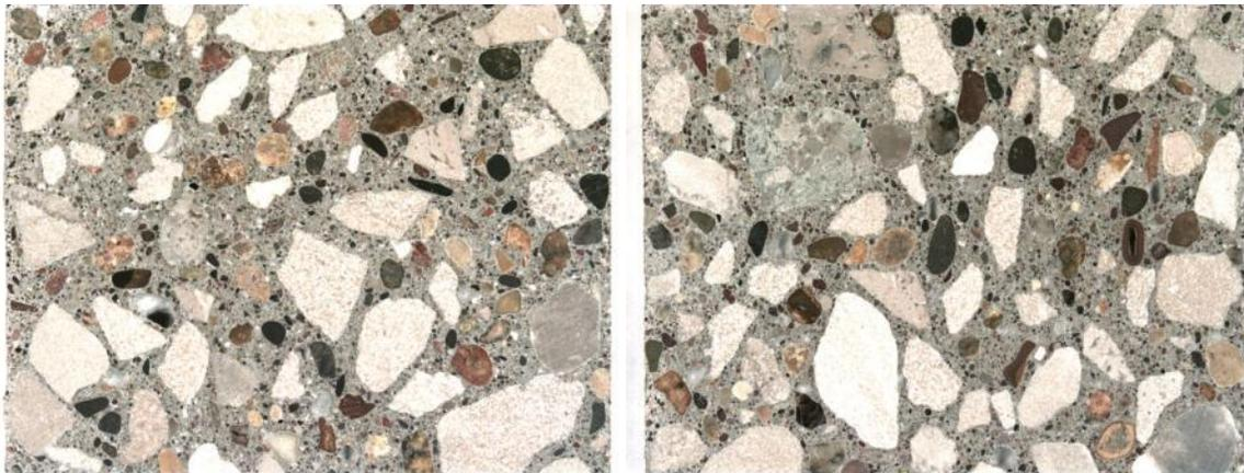
**Figure 9 - Bellevue optical images (no salt) - middle (l), edge (r)**
