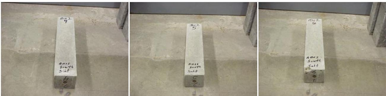
Figure 22 – Army Post Road freeze thaw beams (no salt)
