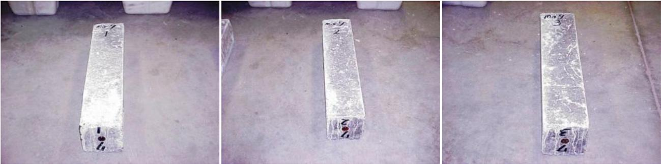
Figure 31 – Bellevue freeze thaw beams (salt)
