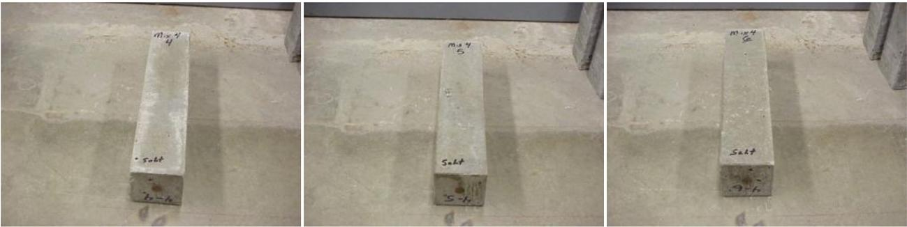
Figure 26 – Woodbine-McCann freeze thaw beams (no salt)
