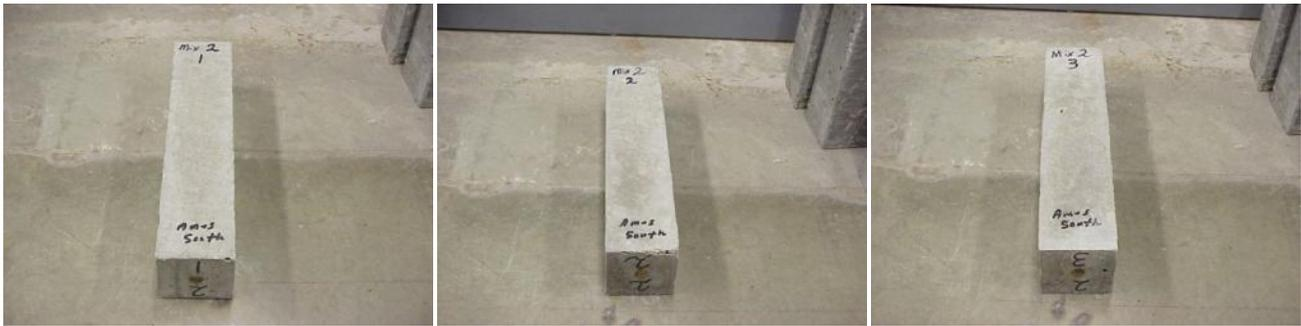
Figure 21 – Ames South freeze thaw beams (salt)
