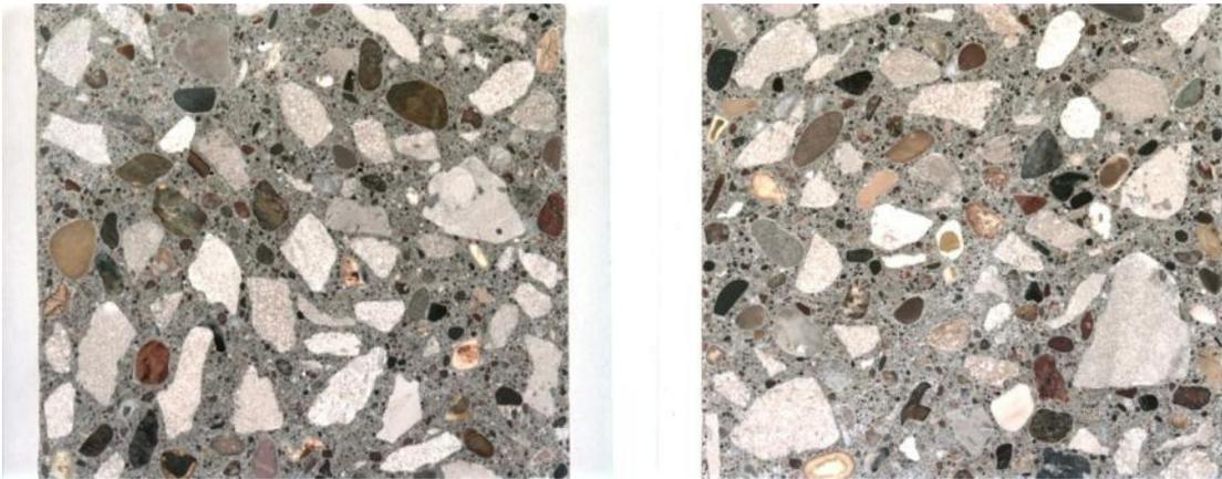
**Figure 6 - Army Post Road optical images (salt) - middle (l), edge (r)**
