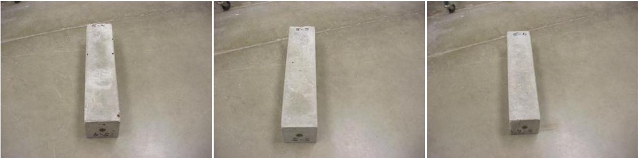
Figure 28 – Anthon freeze thaw beams (no salt)
