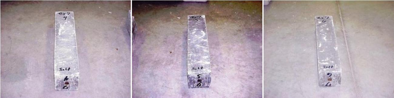
Figure 32 – Turner freeze thaw beams (no salt)
