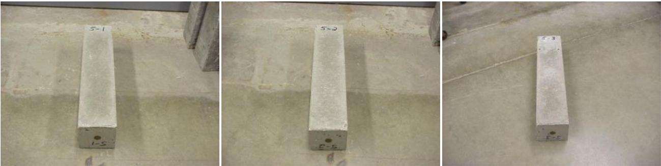
Figure 27 – Woodbine-McCann freeze thaw beams (salt)
