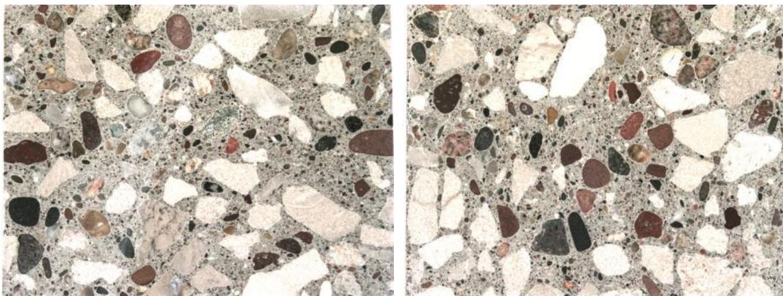
**Figure 10 - Bellevue optical images (salt) - middle (l), edge (r)**
