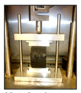
Indirect tensile strength test setup
