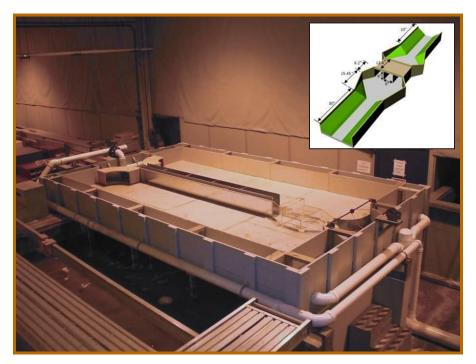
Laboratory hydraulic model and schematic of channel (insert) with three-barrel culvert geometry
