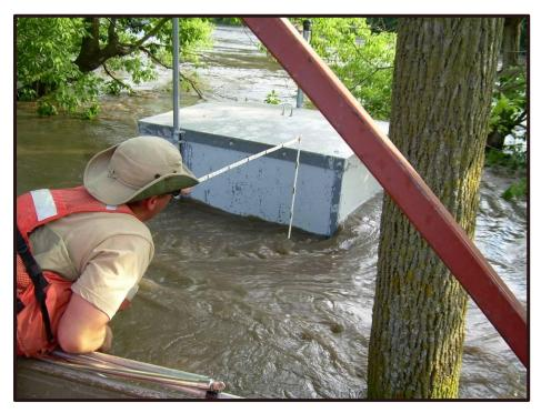
U.S. Geological Survey measures the high water mark on the Cedar River at the Janesville stream gage on June 10, 2008. The record discharge for this site was set that day with streamflow measured at 53,400 cfs.
