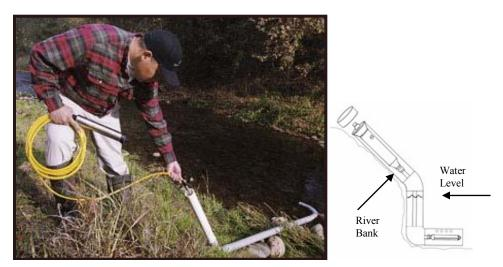
Installation of Water Level Loggers (left) and drawing (right) of Logger Placement
