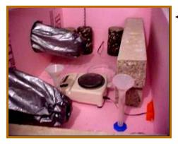
Test chamber measures the freezing characteristics of Calcium Chloride brine.
