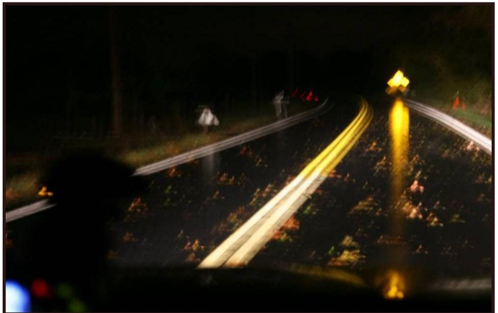
Wet, dark conditions present special challenges to drivers, such as color variations (shown here between two different centerline pavement marking products used on a rural two-lane roadway). In dry conditions, both products are yellow. However, under wet conditions the nearer product appears white in color (like edge line markings) which is an obvious safety concern.
