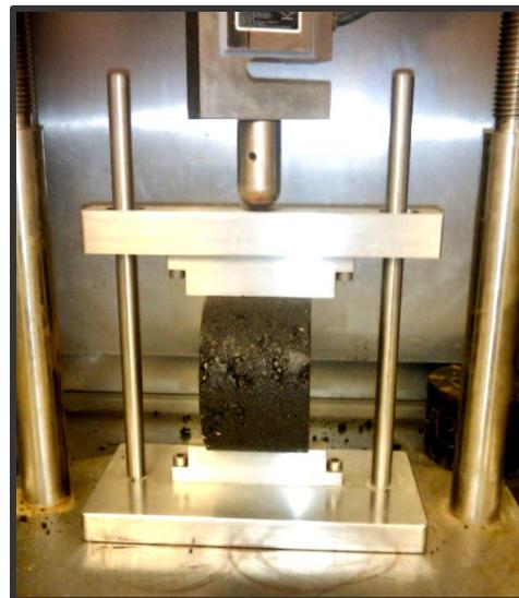
Indirect tensile strength test setup
