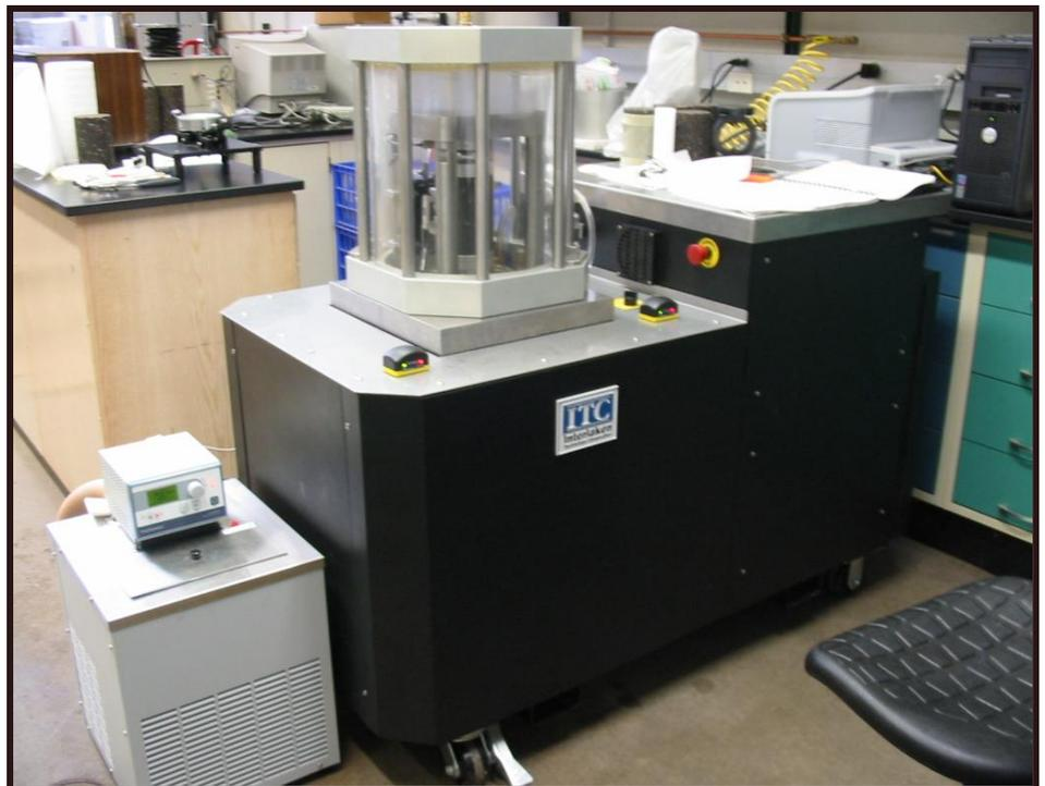
CIR-emulsion mixtures tested using an Interlaken Gyrotory Compactor
