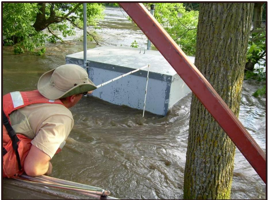
U.S. Geological Survey measures the high water mark on the Cedar River at the Janesville stream gage on June 10, 2008. The record discharge for this site was set that day with streamflow measured at 53,400 cfs.
