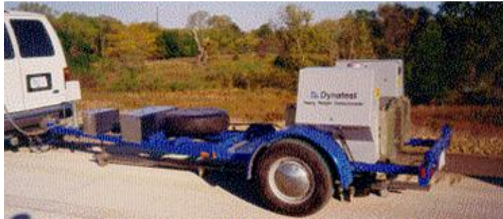
Figure 3. Falling Weight Deflectometer
