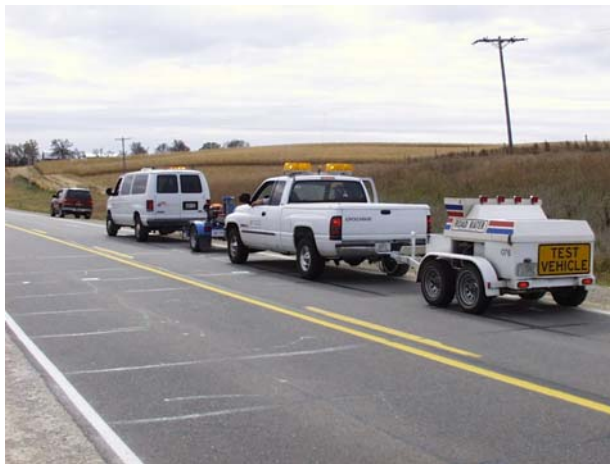
Figure 4. Measuring deflections with FWD and Road Rater
